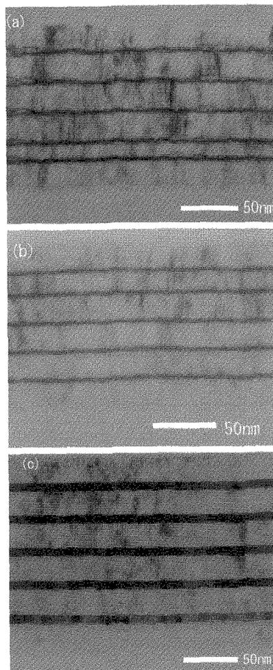
Fig.2. Cross-section TEM bright field image from annealed CoPt/AlN multilayer; thickness of CoPt layer is (a) 1 nm, (b) 2 nm, (c) 8 nm.
