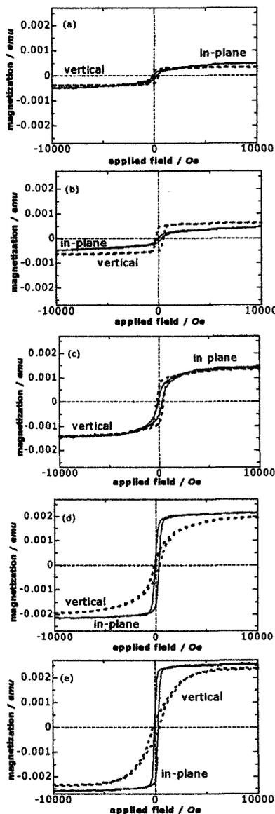
Fig.3. Magnetic hysteresis loops of annealed CoPt/AlN multilayer films; thickness of CoPt layer is (a) 1 nm, (b) 2 nm, (c) 4 nm, (d) 6 nm and (e) 8 nm.
