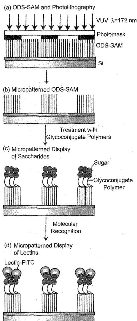
Figure 1 Schematic illustration of micropatterned display: (a) photolithography on ODS-SAM, (b) micropatterned ODS-SAM, (c) micropatterned display of carbohydrate, and (d) micropatterned display of lectin.
