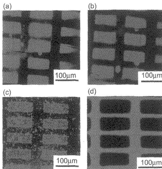
Figure 7 Fluorescence micrographs on Si substrate: (a) Con A on 1-coated ODS-SAM, (b) Con A on 2-coated ODS-SAM, (c) RCA<sub>120</sub> on 3-coated ODS-SAM, and (d) RCA<sub>120</sub> on 4-coated ODS-SAM (negative pattern).
