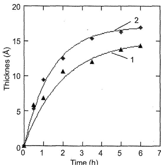
Figure 3 Thicknesses of the glyco-polymers (1 and 2) of ODS-SAM on Si substrate estimated by ellipsometry: (-) calculation according to Langmuir isotherms.
