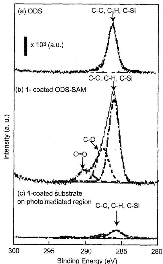
Figure 5 XPS spectra on Si substrate: (a) ODS-SAM, (b) 1-coated ODS-SAM, and (c) 1-coated substrate on photoirradiated region.
