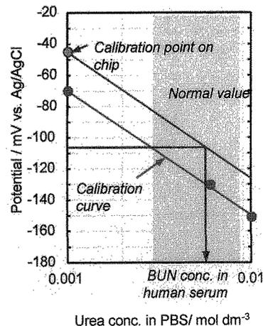
Fig.7 Calibration curves of BUN sensor for practical use.
