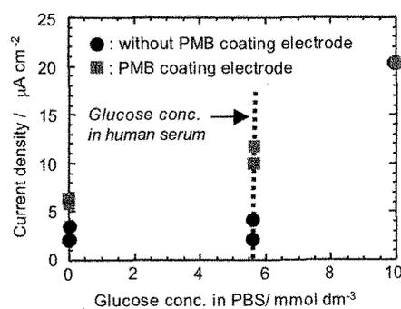
Fig.5 Effect of biocompatible treatment on micro-glucose sensor using PMB.
