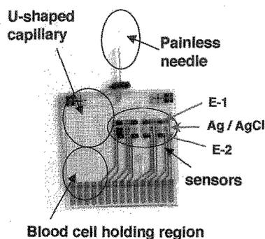
Fig.1 Photograph of disposable healthcare chip.
