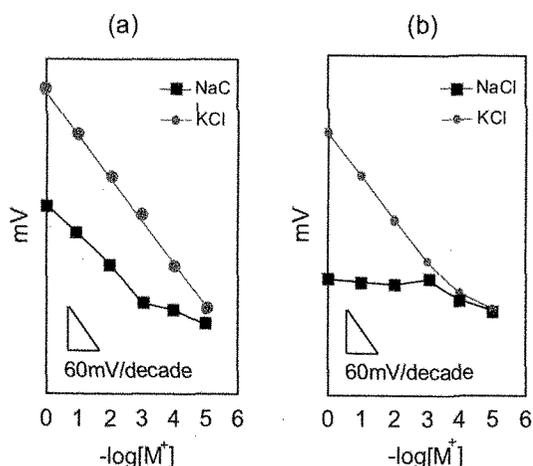
Fig. 3 Calibration curves for  $\text{K}^+$  sensors; (a) ionophore:anion-exclusion-agent=1:1, (b) ionophore:anion-exclusion-agent=1:0.5, respectively.
