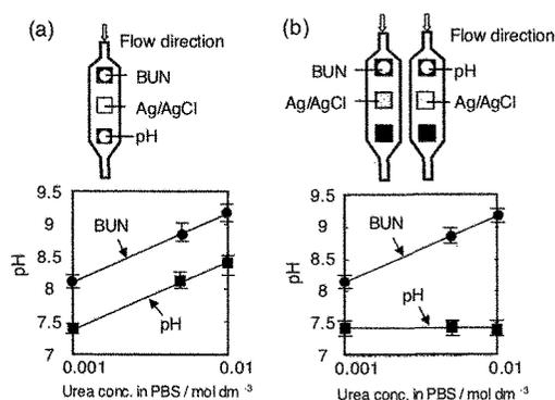
Fig.6 Controlling of mutual interference using branch channel. (a) BUN and pH sensors are set in the single channel, (b) BUN and pH sensors are set in the branch channel.
