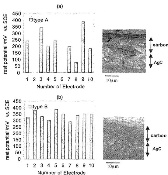
Fig.2 Evaluation of stability in 10 carbon electrodes, and cross sectional SEM images of each typical carbon electrode. Type A electrode consists of large graphite particle, type B electrode consist of small grains.
