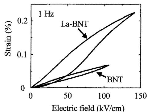
Fig.5 Electric-field-induced strain of the ceramics.
