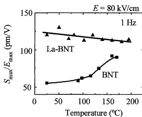
Fig.6  $S_{\text{max}}/E_{\text{max}}$  property of the ceramics.
