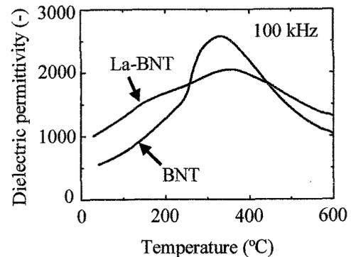
Fig.2 Dielectric permittivity as a function of temperature of the ceramics.
