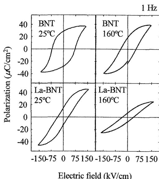
Fig.4  $P$ - $E$  hysteresis loops of the ceramics at 25°C and 160°C.
