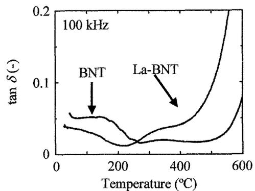
Fig.3 Dielectric loss property as a function of Temperature of the ceramics.
