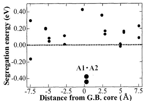
Fig. 6. Segregation energy versus distance from grain boundary core to the each substitution sites. Below dotted line, grain boundary segregation is energetically favorable.
