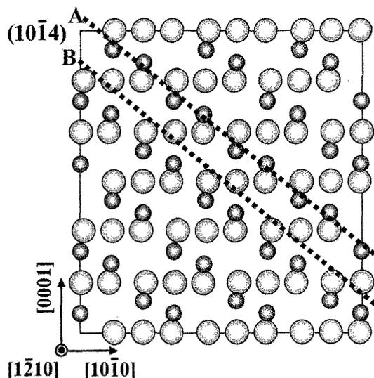
Fig. 1. Crystal structure of  $\alpha\text{-Al}_2\text{O}_3$  viewed from  $[12\ 10]$  directions. Large and small circles represent oxygen and aluminium atoms, respectively. The dashed lines mark the two terminated planes, A: Al-terminated and B: O-terminated plane.
