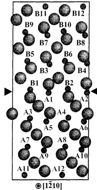
Fig. 5. Substitution sites of Lu atoms in the Al-terminated grain boundary supercell.
