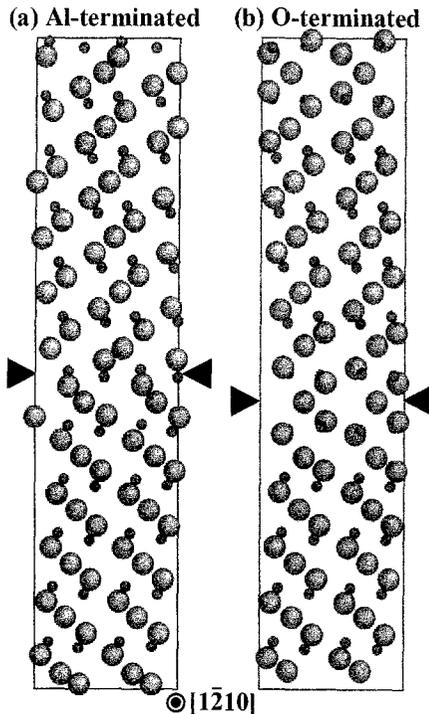
Fig. 4. Relaxed stable atomic structures of (a) Al-terminated and (b) O-terminated grain boundary viewed along  $[1\bar{2}10]$  direction.
