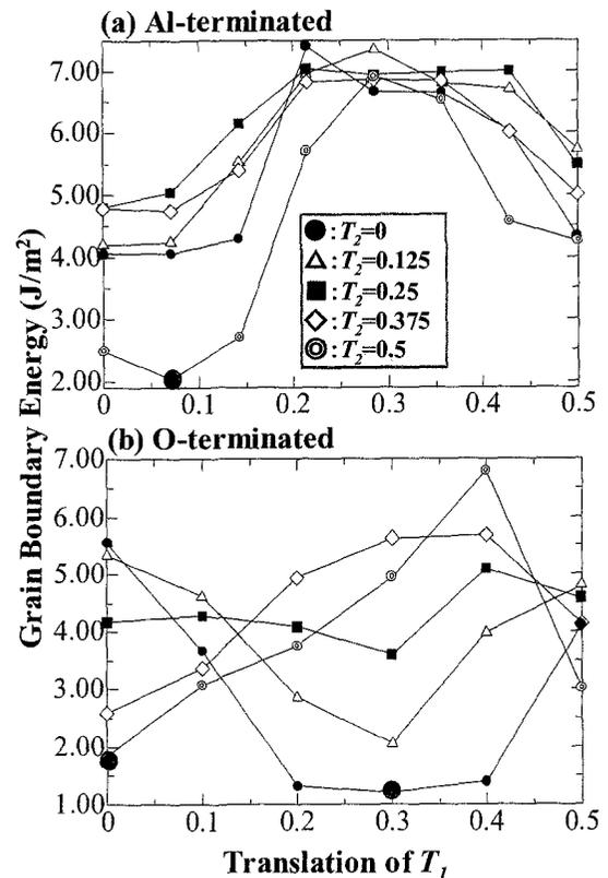
Fig.3. Calculated grain boundary energies with (a) Al-terminated and (b) O-terminated structures versus rigid-body translation of  $T_1$  and  $T_2$ . The lowest energies states are indicated by the large dotted circles.
