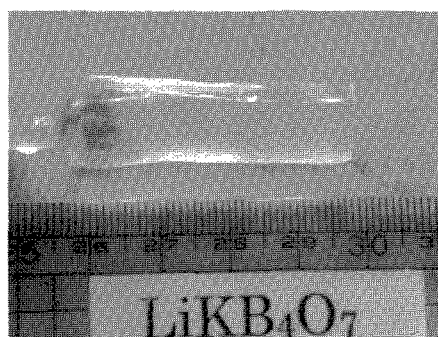
Fig.6 high-quality as-grown \text{LiKB}_4\text{O}_7 crystal
