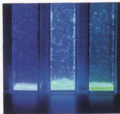
Figure 3. Original CdS flocculants (c) and the nanocrystals photoetched at 457.9 nm (a) and 476 nm (b).
