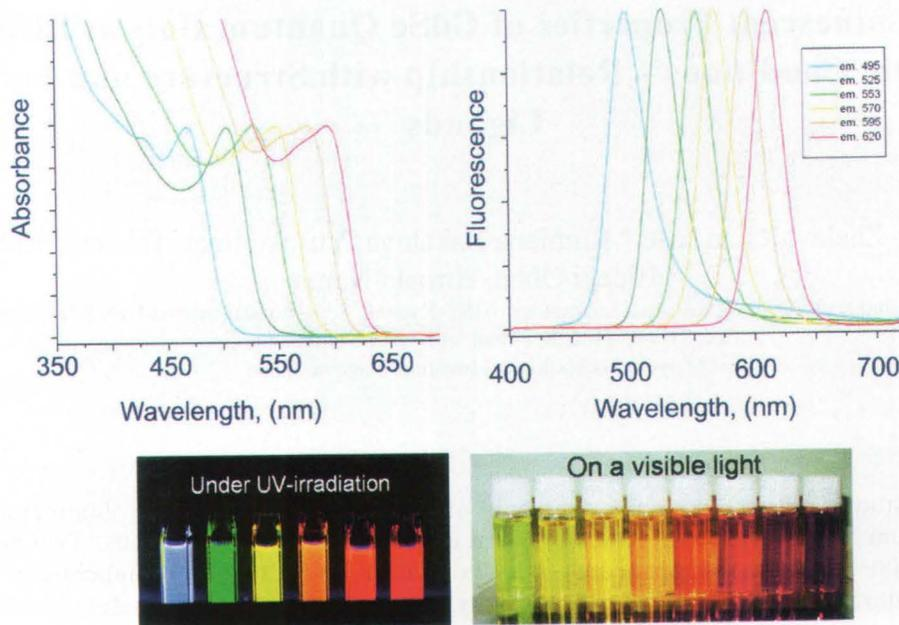
Fig. 1. Spectral characteristics of CdSe quantum dots synthesized at high temperature (120-280 °C, from blue to red color) at Cd:Se ratio 1:1.
