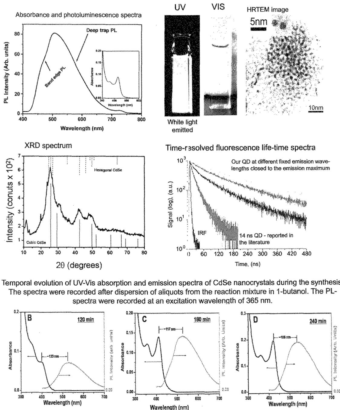
Fig. 3. Spectral characteristics and HRTEM images of CdSe QDs synthesized at room temperature at Cd:Se ratio 1:1.
