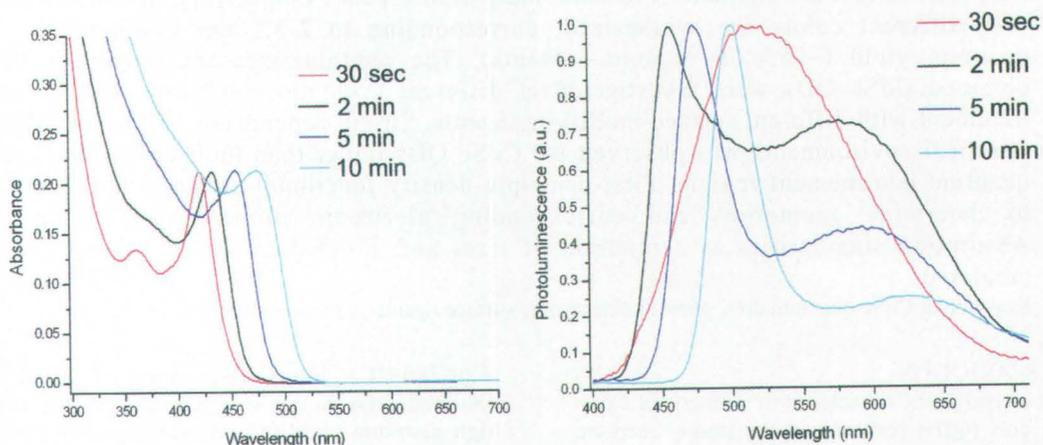
Fig. 2. Spectral characteristics of CdSe QDs synthesized at high temperature (150 °C) in excess of selenium (Cd:Se = 1:4).
