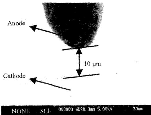
Fig.2 SEM image of the anode and cathode
