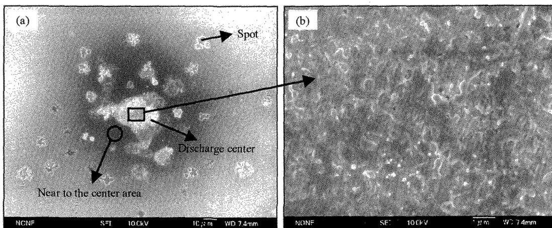
Fig.5 FESEM images of cathode surface after 5 s deposition of discharge when gap was 50 µm and pressure was 100 kPa
