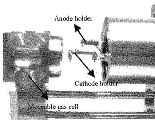
Fig.1 Microplasma discharge cell in SEM
