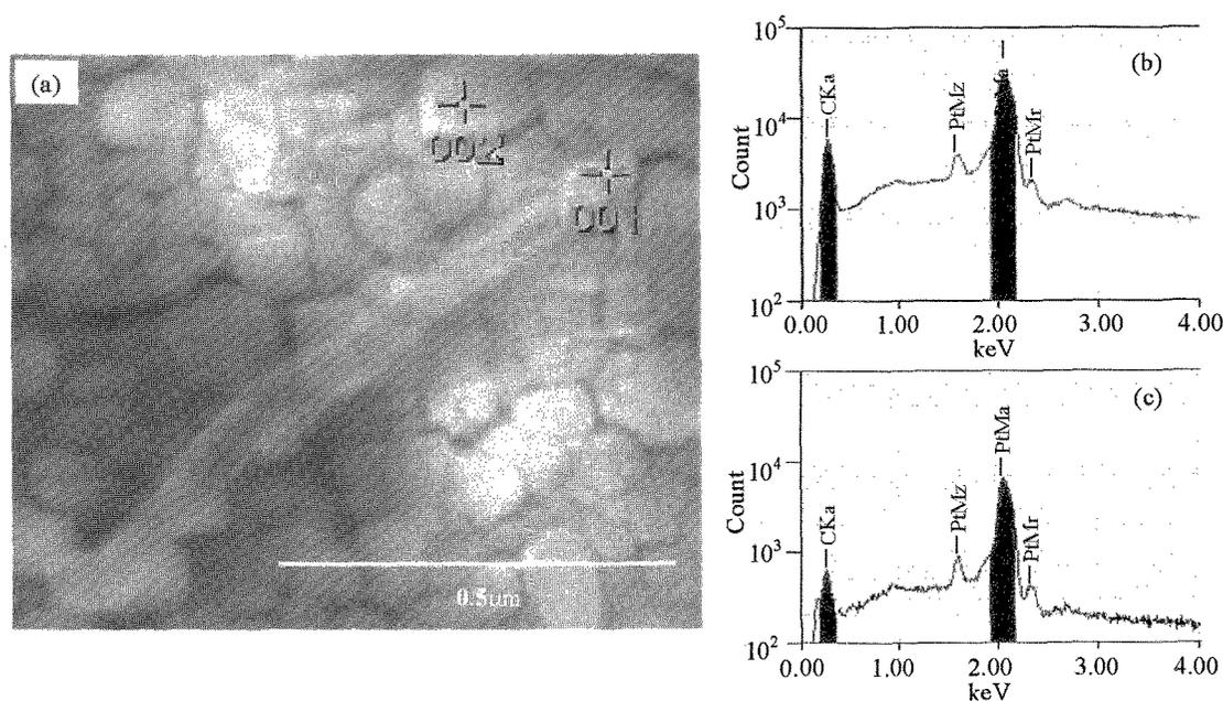
Fig.7 EDX of cathode surface after 5 s operation of discharge when gap was 50  $\mu\text{m}$  and pressure was 100 kPa
