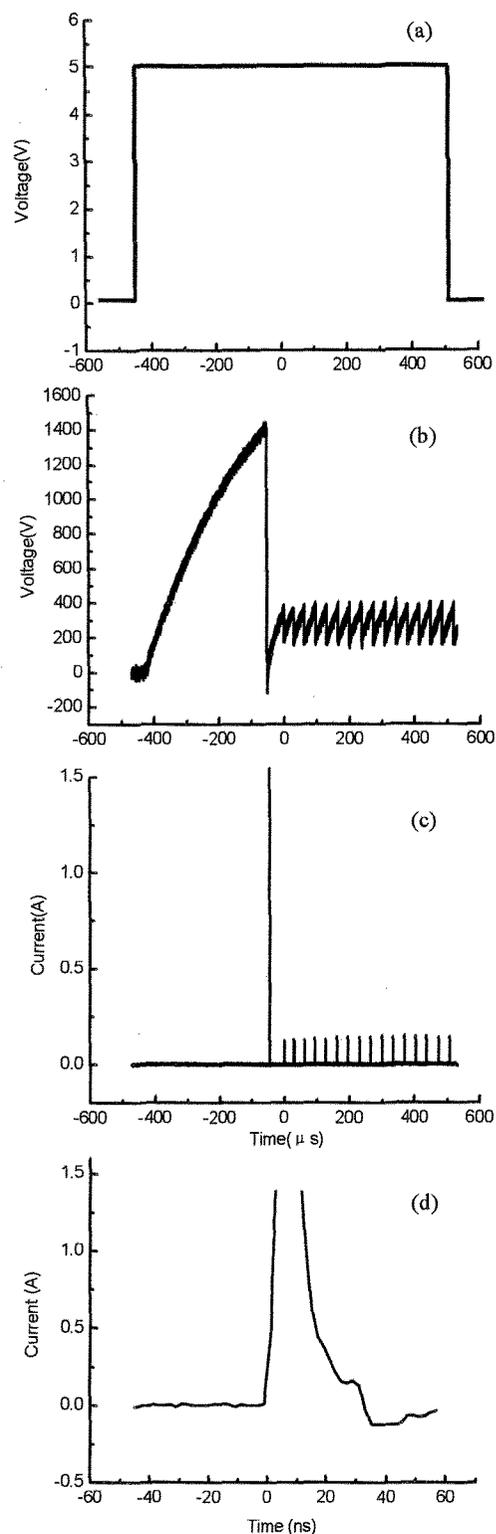
Fig.4 Voltage and current waveforms for the  $\text{CH}_4$  100 kPa pressure and 50  $\mu\text{m}$  gap gas discharge (a) Applied pulse high voltage, (b) Anode monitored voltage, (c) Cathode current, (d) Current of the initial discharge in a pulse on the expanded time
