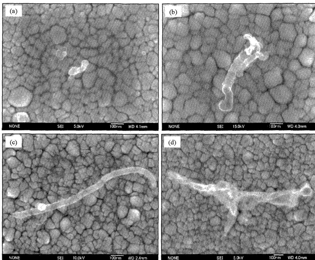
Fig.6 FESEM images of cathode surfaces after different time operation discharge when gap was 50 µm and pressure was 100 kPa (a) 1 s, (b) 3 s, (c) 5 s and (d) 10 s
