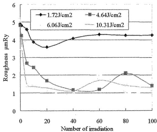
Fig. 5 Surface roughness at different number of irradiation shots
