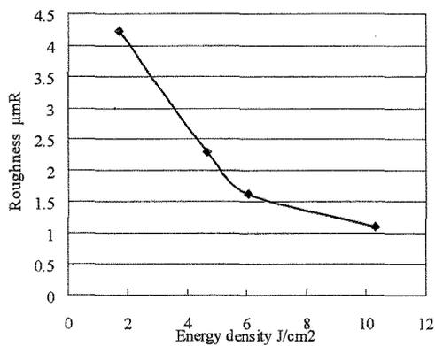
Fig. 4 Surface roughness vs. energy density of E-beams
