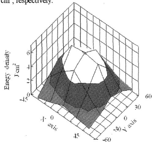
Fig. 3 Energy density distribution of one irradiation shot
