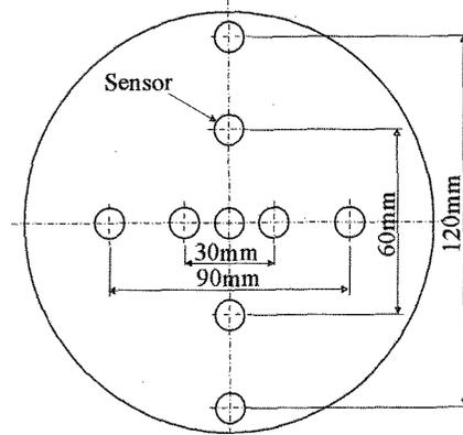
Fig. 2 The structure of calorimeter of measuring energy density of electron beams
