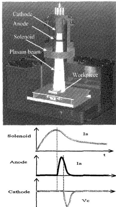
Fig. 1 A schematic illustration of high current high enthalpy plasma machine
