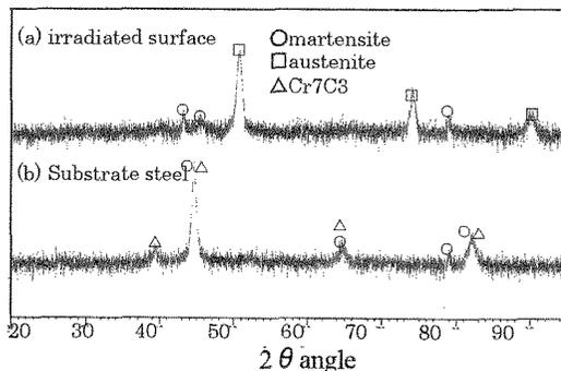
Fig. 9 X-ray diffraction profile (a) EB irradiated surface (b) Substrate steel (ground surface)
