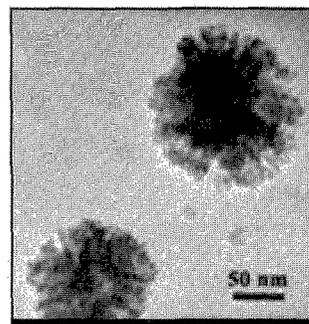
Fig. 4 TEM image of Py-g-PEG2k.5(19.7%) micelles. The polymer concentration was 0.1 mg / ml.
