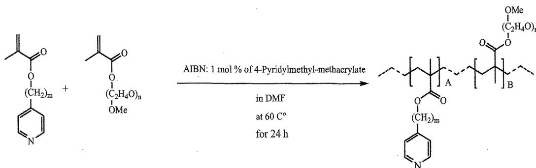
Scheme 1 Copolymerization of Methyl-Terminated PEG Macromonomers with 4-Pyridylmethyl Methacrylates.
