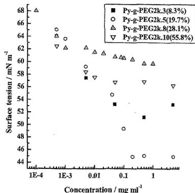
Fig. 3 Surface tension as a function of concentration for Py-g-PEG2k.x (x=3(8.3%), 5(19.7%), 10(55.8%).
