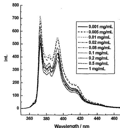
Fig. 5 Fluorescence emission spectra ( $\lambda_{ex} = 339$  nm) of pyrene ( $6 \times 10^{-5}$  M) in the presence of various concentrations of Py-g-PEG2k.5(19.7%).
