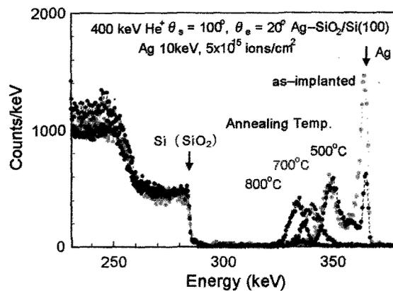
Fig. 3. HRBS yields of Ag-implanted SiO<sub>2</sub>/Si samples before and after annealing at various temperatures of 500°C, 700°C and 800°C.
