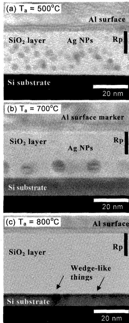
Fig. 5. Cross-sectional TEM images of Ag-implanted 25-nm- $\text{SiO}_2$  layers on Si samples at 10 keV with  $5 \times 10^{15}$  ion/ $\text{cm}^2$  after annealing at various temperatures of (a)  $500^\circ\text{C}$ , (b)  $700^\circ\text{C}$  and (c)  $800^\circ\text{C}$ .
