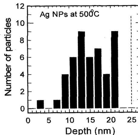
Fig. 6. Histogram of Ag NPs formed in 25-nm- $\text{SiO}_2$  layers after annealing at  $500^\circ\text{C}$  (from Fig. 5(a)).
