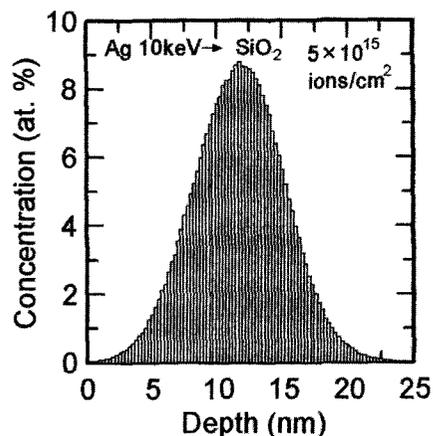
Fig. 2. Estimated concentration of Ag atoms implanted into SiO<sub>2</sub> medium at 10 keV with 5 × 10<sup>15</sup> ions/cm<sup>2</sup> calculated by TRIM-DYN program.
