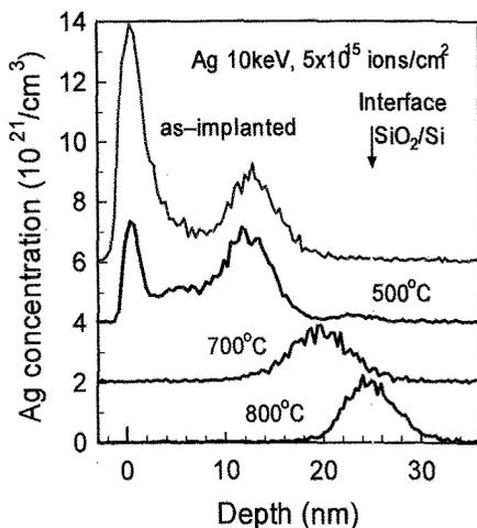
Fig. 4. Depth profiles of Ag atoms implanted  $\text{SiO}_2$  layer before and after annealing at various temperature of  $500^\circ\text{C}$ ,  $700^\circ\text{C}$  and  $800^\circ\text{C}$  by HRBS data (from Fig. 3).
