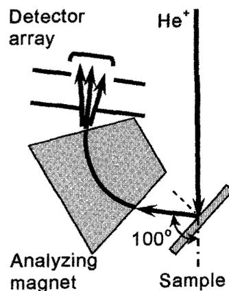
Fig. 1. Schematic configuration of a measurement system for high-resolution Rutherford back-scattering spectrometry (HRBS).
