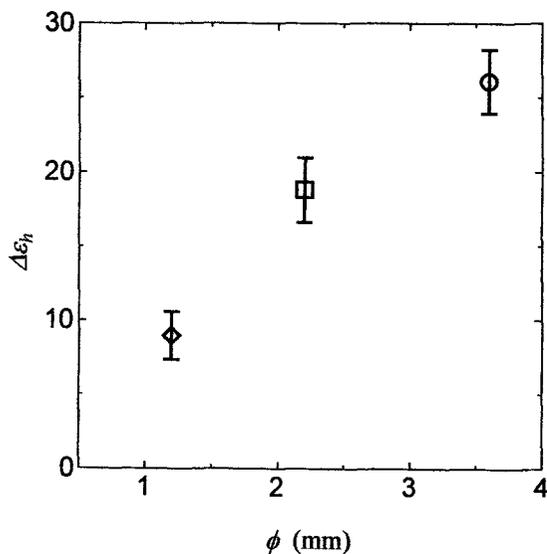
Fig.6 Plot of the relaxation strength for free water at forearm flexor against the outer diameters of outer conductor of electrodes.
