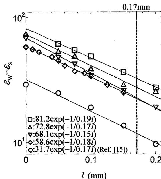
Fig.2 Plots of  $\epsilon_w - \epsilon_s(l)$  against  $l$  with the lines drawn by least square fitting of exponential function given by eq.(2). The measurements were performed five times.
