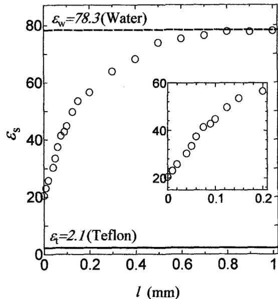
Fig.1 Plot of the static dielectric constant against the distance between surfaces of Teflon and electrode.
