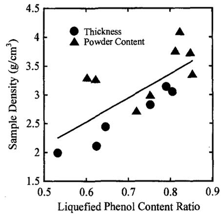
Fig.2 Relationship between liquefied phenol content ratio and sample density.
