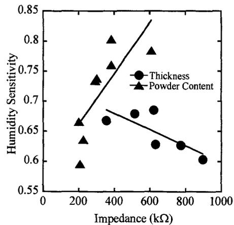
Fig.3 Impedance dependence of humidity sensitivity.
