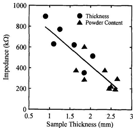
Fig.1 Sample thickness dependence of impedance. Circles and triangles are represented the results for the samples with various thicknesses and with various paper powder contents, respectively.
