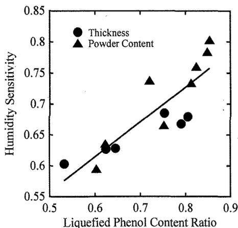
Fig.4 Relationship between humidity sensitivity and liquefied phenol content. ratio
