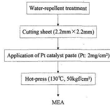
Fig. 6. Manufacturing procedure of MEA.
