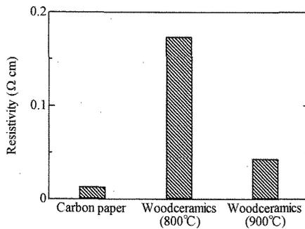
Fig. 5. Resistivity of woodceramics sheet.
