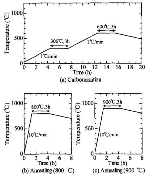
Fig. 3. Temperature changes in carbonization and annealing.
