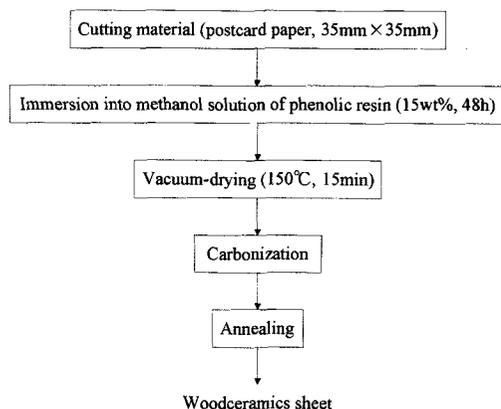
Fig. 2. Outline of manufacturing procedure for woodceramics sheet.
