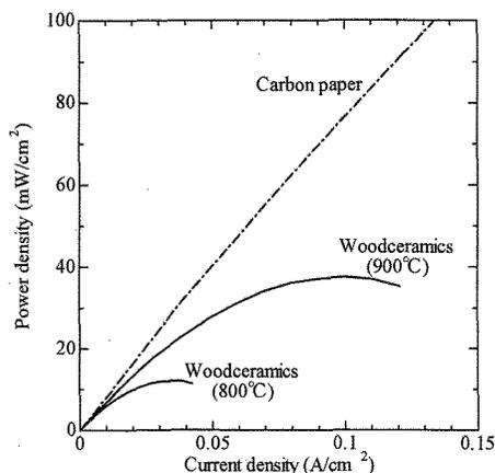
Fig. 9. Power density-current density characteristics.
