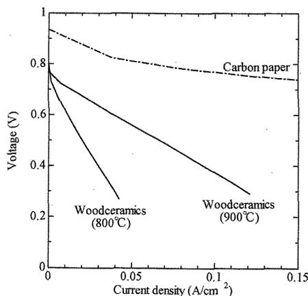
Fig. 8. Voltage-current density characteristics.
