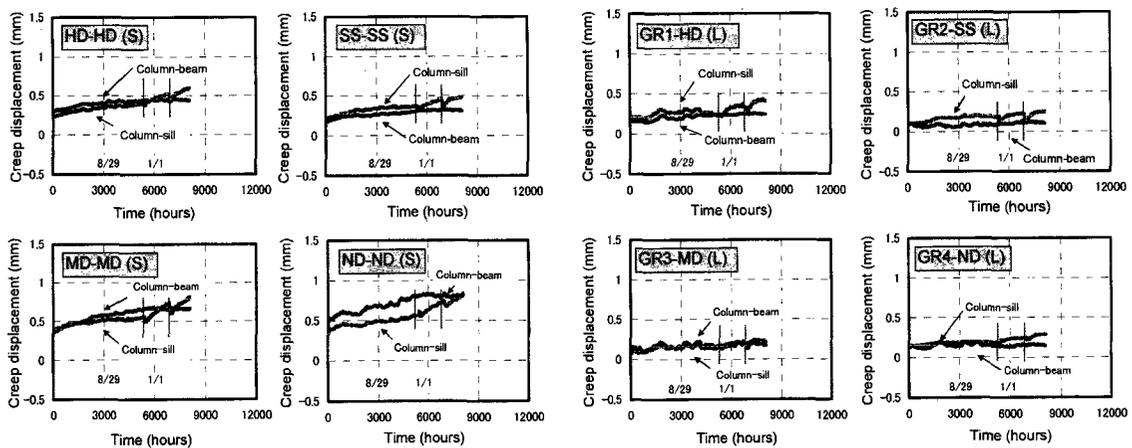
Fig.5. Changes of compression creep displacement perpendicular to the grain of column-and-sill joints (CAS-joints).
