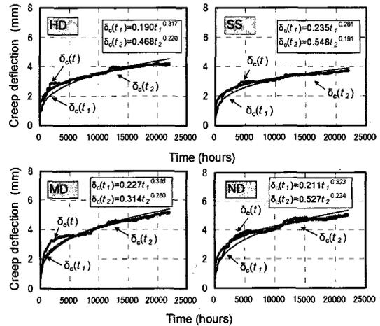
Fig. 4. Comparisons between  $\delta_c(t)$  and  $\delta_c(t_1)$  or  $\delta_c(t_2)$  for HD, SS, MD and ND.
