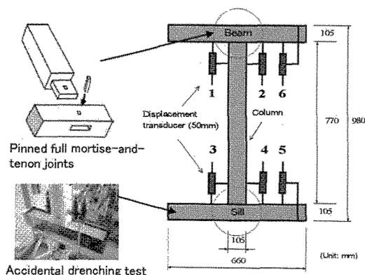
Fig. 1. The shape and size of column-and-sill joints (CAS-joints) and the setting positions of displacement transducers.
