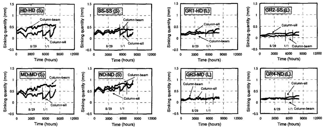
Fig. 6. Changes of sinking quantity, which means sum of the creep displacement and the contraction or swelling of sills, of CAS joints.
