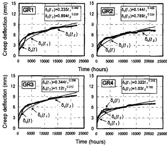
Fig. 3. Comparisons between measured creep deflections [ $\delta_c(t)$ ] and creep deflections calculated by power law [ $\delta_c(t_1)$ ,  $\delta_c(t_2)$ ] for GR1, GR2, GR3 and GR4.
