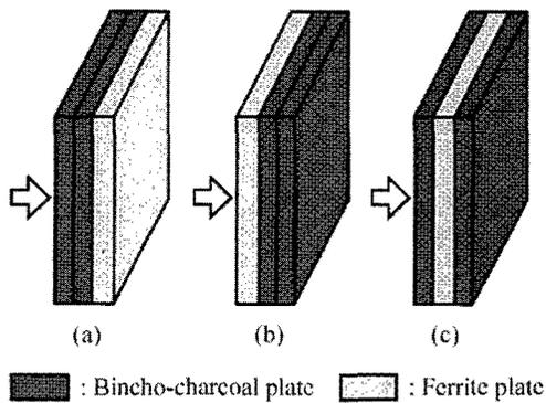
Fig. 2. Sketch of the geometry of three different compound plates. (a), (b), and (c) are the sample A, sample B, and sample C, respectively.
