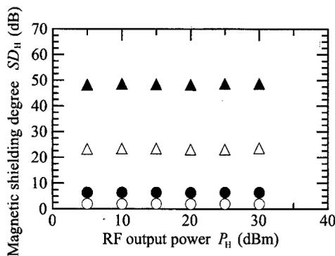
Fig. 5. Typical characteristics of  $SD_H$  for the single bincho-charcoal plate as functions of RF output power  $P_H$ . The open circles, solid circles, open triangles, and solid triangles represent the result for 2 MHz, 20 MHz, 200 MHz, and 2 GHz, respectively.
