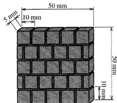
Fig. 1. Sketch of the geometry of a typical bincho-charcoal plate.
