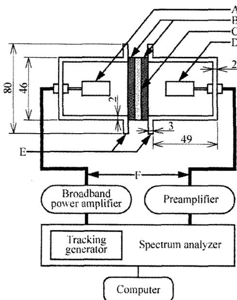
Fig. 3. Schematic diagram of the experimental arrangement used to measure the electromagnetic shielding characteristics for the compound plate. Here, A represents the transmitting antenna, B the bincho-charcoal plate, C the ferrite plate, D the receiving antenna, E the metal cell, and F the coaxial cable.
