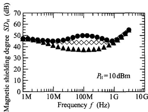
Fig. 7. Distributions of the RF magnetic shielding degree  $SD_H$  for the three different compound plates as functions of frequency  $f$ , under constant RF output power  $P_H$  (10 dBm) of the transmitting antenna. The solid triangles, open diamonds, and solid circles represent the samples A, B, and C, respectively.
