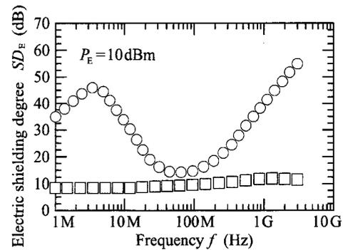
Fig. 6. The RF electric shielding degree  $SD_E$  for the single bincho-charcoal and ferrite plates as functions of frequency  $f$ . The open circles and open squares represent the single bincho-charcoal and ferrite plates, respectively.
