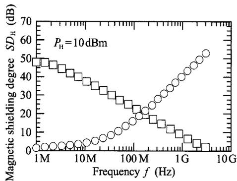
Fig. 4. RF magnetic shielding degree  $SD_H$  for the single bincho-charcoal and ferrite plates as functions of frequency  $f$ . The open circles and open squares represent the single bincho-charcoal and ferrite plates, respectively.
