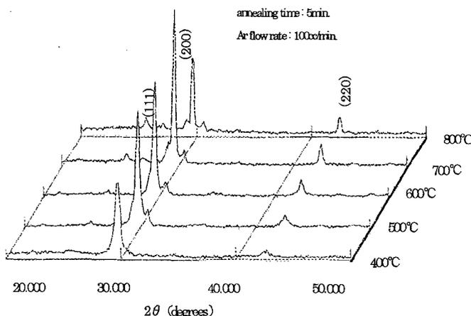
Fig. 4 (a) XRD peaks in the case of annealing time of 5 minutes.
