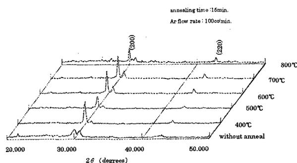
Fig. 6 (a) XRD peaks in the case of annealing time of 15 minutes.
