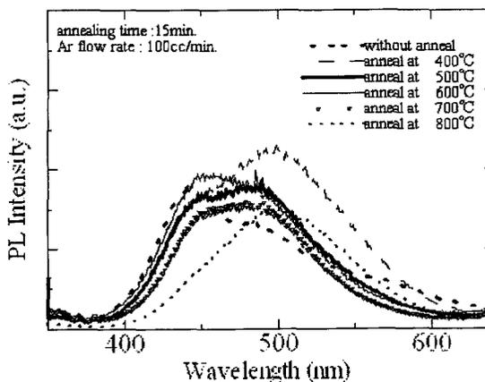
Fig. 6 (b) PL properties in the case of annealing time of 15 minutes..
