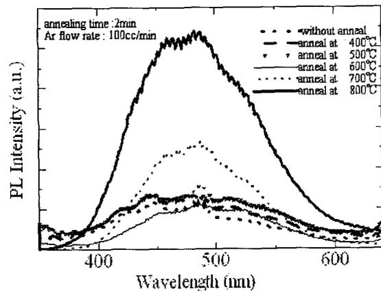
Fig. 3 (b) PL properties in the case of annealing time of 2 minutes.
