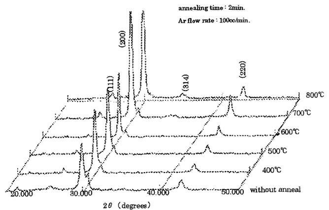
Fig. 3 (a) XRD peaks in the case of annealing time of 2 minutes.
