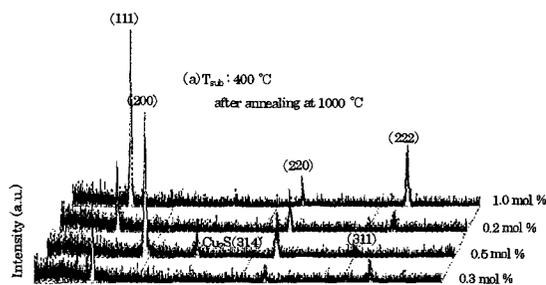
Figure 2(b) XRD spectrum of SrS:Cu films.
