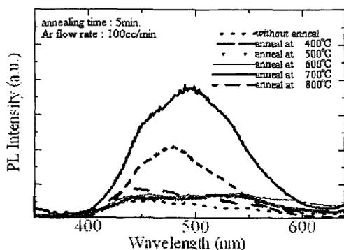
Fig. 4 (b) PL properties in the case of annealing time of 5 minutes..
