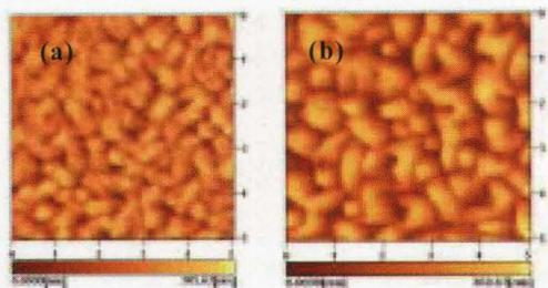
Fig. 3: AFM images of as-deposited BIT thin films with (a)  $\text{TiO}_2$  anatase layer and (b) no-layer.
