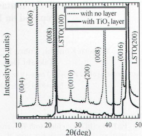
Fig. 2: XRD patterns of as-deposited BIT thin films with  $\text{TiO}_2$  anatase layer and no-layer.
