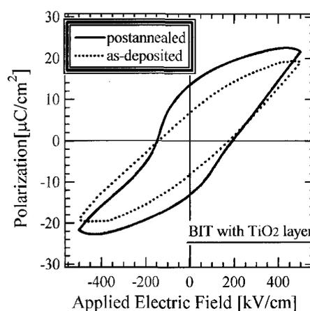
Fig.6:  $P$ - $E$  hysteresis loops of as-deposited (dashed line) and postannealed (solid line) BIT thin films with  $\text{TiO}_2$  anatase layer.
