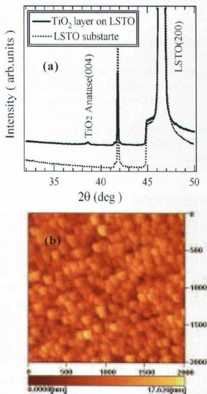
Fig. 1: (a) XRD pattern of  $\text{TiO}_2$  anatase thin film (solid line) prepared on LSTO substrate. As reference, the XRD pattern of LSTO substrate is also shown as dashed line. (b) AFM image of  $\text{TiO}_2$  anatase thin film prepared on LSTO substrate.
