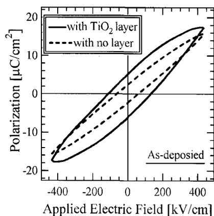
Fig. 4:  $P$ - $E$  hysteresis loops of as-deposited BIT thin films with  $\text{TiO}_2$  anatase layer (solid line) and no-layer (dashed line).
