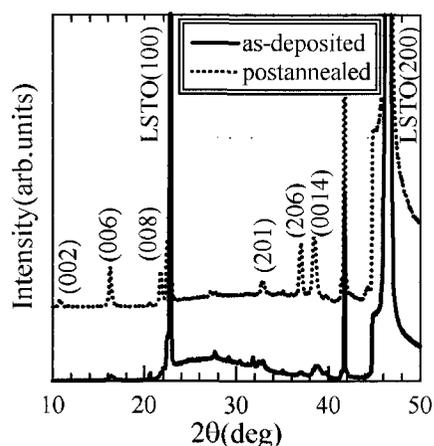
Fig.5: XRD patterns of as-deposited (solid line) and postannealed (dashed line) BIT thin films with  $\text{TiO}_2$  anatase layer.
