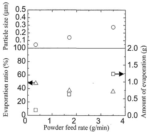
Fig. 2 Particle size, amount of evaporation, and evaporation ratio of the raw material for three different powder feed rates.
