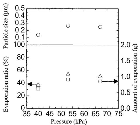
Fig. 4 Particle size, amount of evaporation, and evaporation ratio of the raw material for three different reactor pressures.
