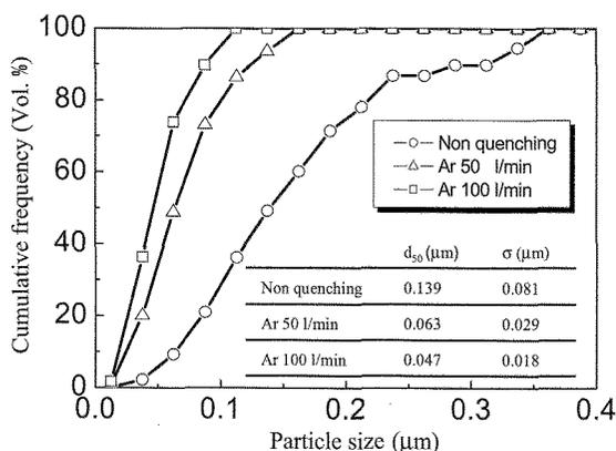
Fig. 6 Size distribution of the copper nanoparticles synthesized with quenching gas of Ar 50, 100l/min in the counter direction of plasma flow.
