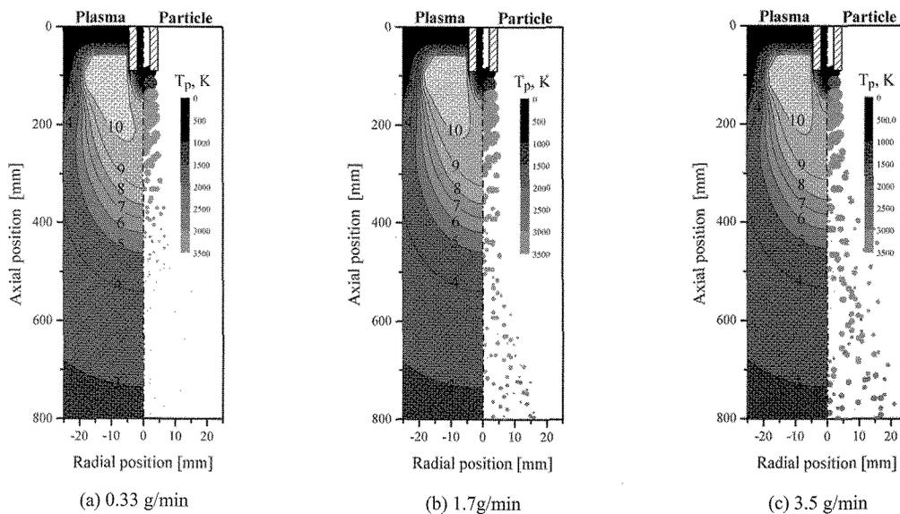
Fig. 1 Numerical analysis of the temperature distribution in the plume (Left,  $\times 10^3$  K), the particle trajectory, the change of in particle size and particle temperature (Right) for three different powder feed rates: (a) 0.33 g/min, (b) 1.7 g/min, and (c) 3.5 g/min.
