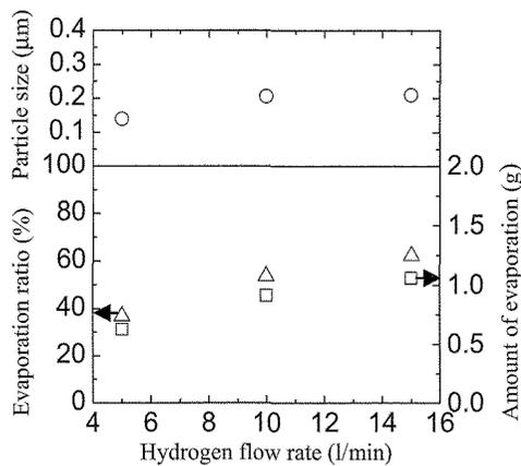
Fig. 3 Particle size, amount of evaporation, and evaporation ratio of the raw material for three different gas flow rates of hydrogen.
