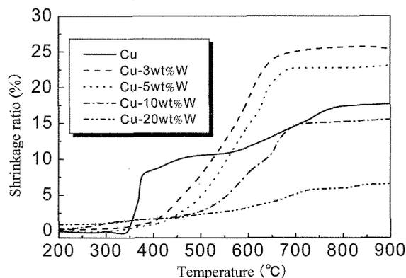
Fig. 7 Thermal shrinkage of Cu–W composite powders.
