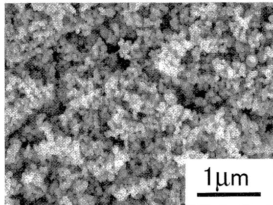
Fig. 5 FE-SEM image of the copper nanoparticles synthesized with quenching gas of Ar 50l/min in the counter direction of plasma flow.
