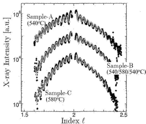
Fig. 9 Measured CTR scattering data (●) and best-fit curves (gray lines) for the three samples. 002 Bragg peaks from GaAs are truncated.
