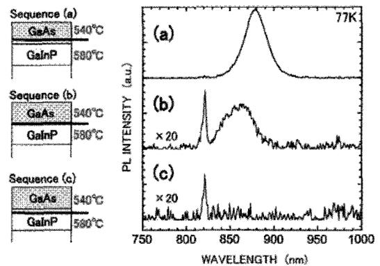
Fig. 4 In the GaAs/GaInP layer growth, the growth temperature was changed from 580°C to 540°C; (a) during the top GaAs growth, (b) just at the interface, and (c) during the GaInP growth. PL from each structure shows a clear answer that the heterointerface should be grown at a lower temperature to eliminate the broad emission.
