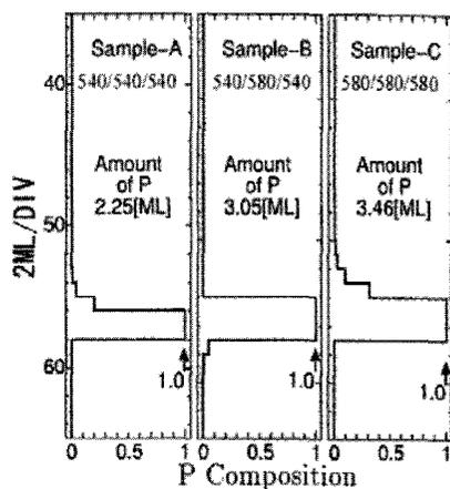
Fig. 11 Obtained P distributions in the three samples. P distributions are much abrupt compared with those of In distributions in the three samples. [After Ref. 26]
