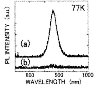
Fig. 3 The broad emission disappeared when the top GaAs was etched off. (a) is PL from the layer structure in Fig. 2 (a). (b) is PL from the layer structure after selective etching of the top GaAs.
