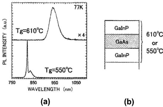
Fig. 1 (a) Photoluminescence spectra from GaInP/GaAs/GaInP structures grown at 610°C and 550°C. (b) Layer structure and growth temperatures. The three layers were grown at the same temperatures, 610°C or 550°C.
