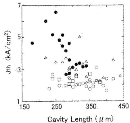
Fig. 6 Threshold currents and heterointerface growth temperatures. ○ the whole layer grown at 540°C. ● the whole layer grown at 580°C. Others contain the low temperature process. [After Ref. 26]
