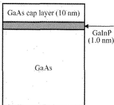
Fig. 7 Sample structure. It is simplified for the measurement convenience but contains the important heterointerface; GaAs on GaInP.
