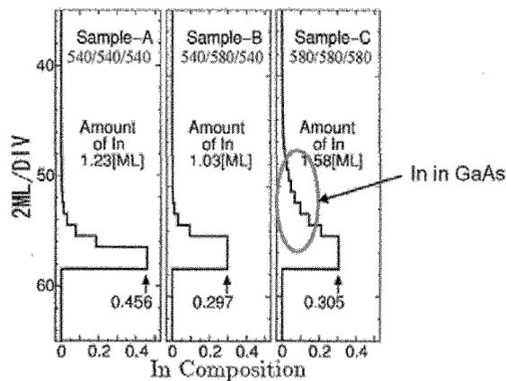
Fig. 10 Obtained In distributions in the three samples. In distribution in the sample-C is much larger and longer than those in the other samples and enough to form GaInAs quantum well in the GaAs layer that can be a recombination center for the broad emission peak. [After Ref. 26]
