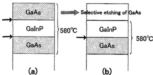
Fig. 2 (a) There are two heterostructures in GaAs/GaInP/GaAs DH. (b) The layers were etched out selectively to find which interface is responsible for the broad emission when the structure is grown at 580°C.
