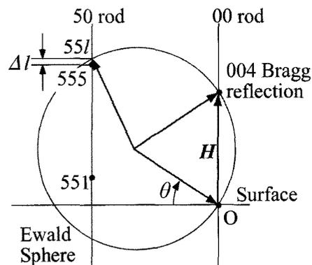
Fig. 1. Illustration of diffraction condition where intensity of CTR scattering is modulated by the excitation of a Bragg reflection. The parameter  $l$  is the momentum transfer perpendicular to the surface, and  $\Delta l$  is the deviation of  $l$  from the 555 Bragg point.
