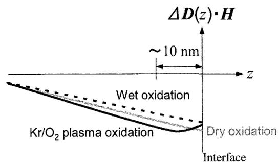
Fig. 4. Depth profiles of strain fields under the  $\text{SiO}_2/\text{Si}$  interfaces, where  $z$  represents the depth and  $\Delta D(z)$  is the sum of displacements defined in Fig. 2. The dotted and gray solid lines correspond to the wet and dry oxidations at  $900\text{ }^\circ\text{C}$ , respectively, and the black solid line does to  $\text{Kr}/\text{O}_2$  plasma oxidation at  $400\text{ }^\circ\text{C}$ .
