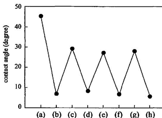
Figure 4 Contact angle measurements of each process of surface modification. (a) GPS-modified substrate; (b, d, f, h) RASDA16 coated substrate by immersing peptide solution; (c, e, g) after sonication.
