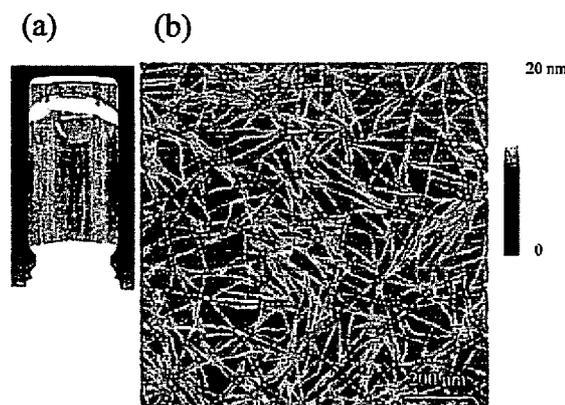
**Figure 1** (a) Photograph of the hydrogel constructed by RASDA16 (0.3 wt%, pH 7.2), (b) AFM image of RASDA16 nanofibers.
