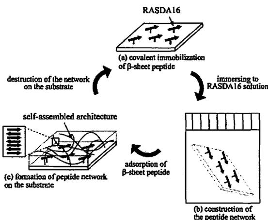
Figure 3 Schematic illustration of re-construction of the peptide network on the substrate.
