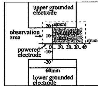
Fig. 3. Cross-sectional view of reactor and observation area of 2D LLS measurements.
