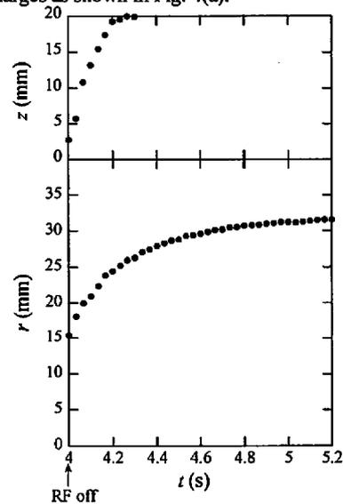
Fig. 7. Trajectories of a position of highest LLS intensity after turning off unmodulated discharge.
