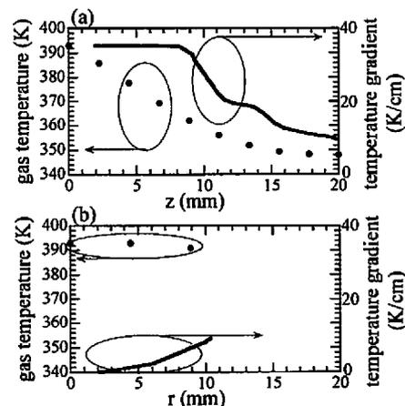
Fig. 8. Spatial profiles of gas temperature and its gradient in z-direction (a) and r-direction (b).
