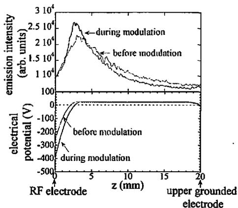
Fig. 10. Spatial profiles of optical emission intensity (a) and time averaged electrical potentials before and during modulation (b).
