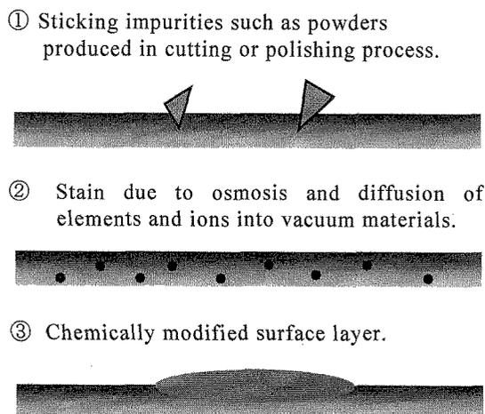
Fig.1 Un-removable impurities, stains and modified surface by a precision cleaning.
