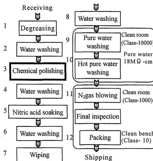
Fig.2 Flow chart of developed chemical polishing and precision cleaning process.
