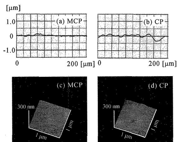
Fig. 3 Surface profiles of the pure titanium samples, (a) MCP and (b) CP, and AFM images of the samples, (c) MCP and (d) CP.
