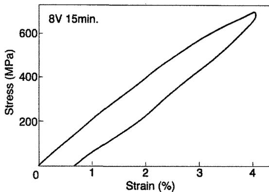
Fig. 9 Stress-strain curve of 8V-15 minutes thin wire.
