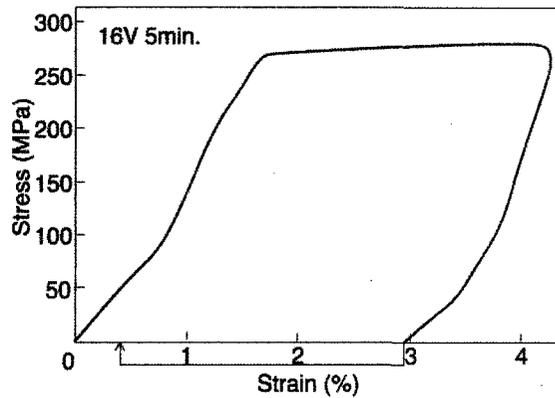
Fig. 11 Stress-strain curve of 16V-5 minutes thin wire.
