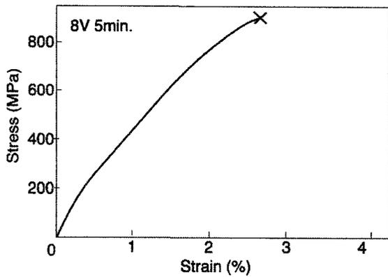
Fig. 8 Stress-strain curve of 8V-5 minutes thin wire.
