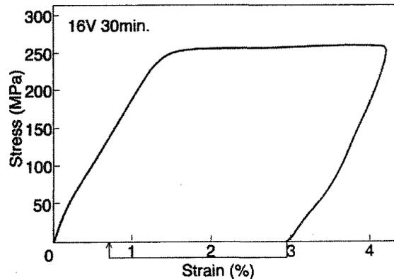
Fig. 13 Stress-strain curve of 16V-30 minutes thin wire.
