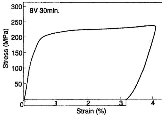
Fig. 10 Stress-strain curve of 8V-30 minutes thin wire.
