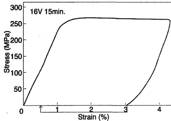
Fig. 12 Stress-strain curve of 16V-15 minutes thin wire.
