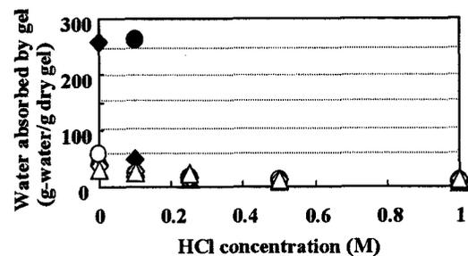
Fig. 3. Water absorption by irradiated CMC gel followed by immersion in HCl for 4 days. ●: 0kGy, ◆: 5kGy, ▲: 10kGy, ○: 20kGy, ◇: 30kGy, △: 50kGy.
