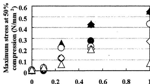
Fig. 5. Maximum stress of gel at 50% compression after immersion in HCl followed by immersion in water. ●: 0kGy, ◆: 5kGy, ▲: 10kGy, ○: 20kGy, ◇: 30kGy, △: 50kGy.
