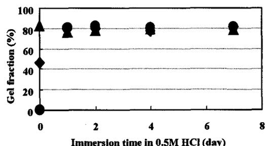
Fig. 2. Gel fraction of irradiated CMC followed by immersion in 0.5M HCl. ●: 0kGy, ◆: 5kGy, ▲: 10kGy.
