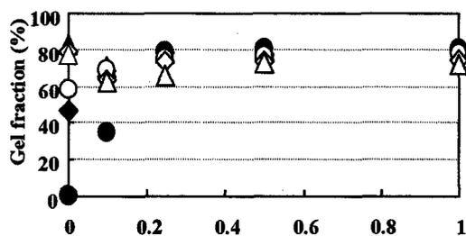
Fig. 1 Gel fraction of irradiated CMC followed by immersion in HCl for 4 days. ●: 0kGy, ◆: 5kGy, ▲: 10kGy, ○: 20kGy, ◇: 30kGy, △: 50kGy.
