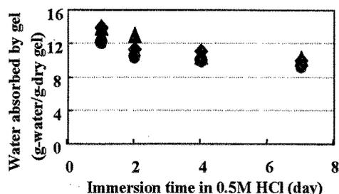
Fig. 4. Water absorption by radiation induced CMC gel followed by immersion in 0.5M HCl. ●: 0kGy, ◆: 5kGy, ▲: 10kGy.
