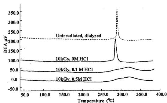
Fig. 9 DTA of unirradiated and irradiated samples at 10kGy followed by immersion in acid.
