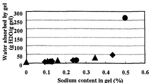
Fig. 7. Relation between sodium content in gel and water absorbed by gel. ●: 0kGy, ◆: 5kGy, ▲: 10kGy.
