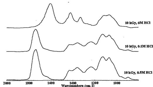
Fig. 8 FT-IR spectra of irradiated samples at 10 kGy followed by immersion in HCl.
