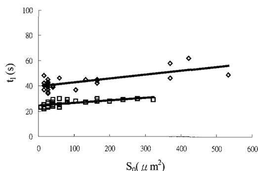
Figure 4. Durations of lag phase  $t_l$  at temperatures of 13.6 °C ( $\diamond$ ) and 47.7 °C ( $\square$ ) for microcapsules with different initial sizes  $S_0$ .
