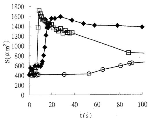
Figure 2. Time courses of cross-sectional area of microcapsules dispersed in ethanol-DOP mixture with various ethanol compositions of  $\circ$ : 30%,  $\blacklozenge$ : 70%,  $\square$ : 100% at  $25^\circ\text{C}$ .
