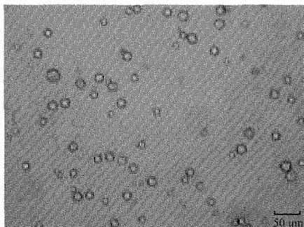
Figure 1. Optical micrographs of microcapsules observed at room temperature.
