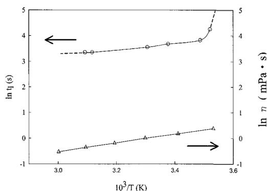
Figure 5. Logarithms of  $t_l$  and viscosity coefficient  $\eta$  of ethanol as a function of reciprocal of absolute temperature.
