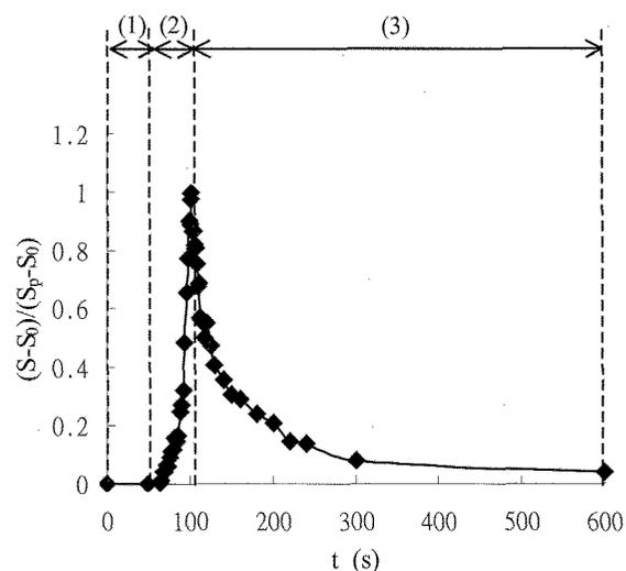
Figure 3. Typical time course of reduced cross-sectional area of microcapsules dispersed in pure ethanol observed at  $50.2^\circ\text{C}$  and the definition of (1) lag phase, (2) swelling phase and (3) shrinking phase.
