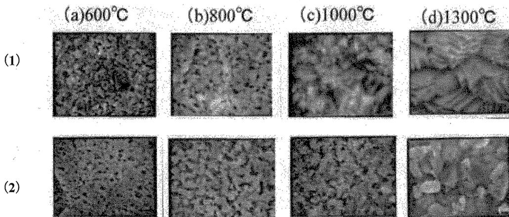
Fig3. SEM photograph of sintered Ni electrode films prepared from 100nm Ni particle size at various temperature (1) without an addition and (2) with an addition of the BT resin.
