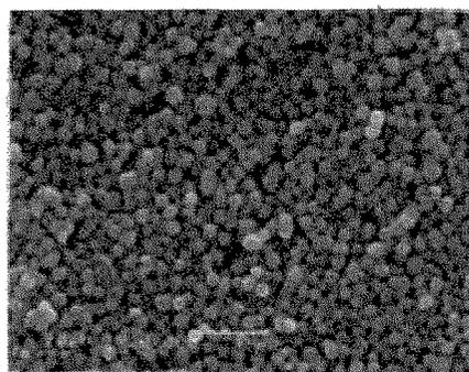
Fig1 SEM image of 100nm Ni powder.
