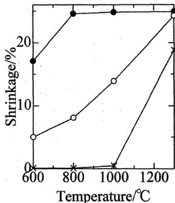
Fig2. relationship between a firing temperature and a shrinkage ● : with no addition of BT resin ○ : addition of BT resin × : Dielectric green sheet
