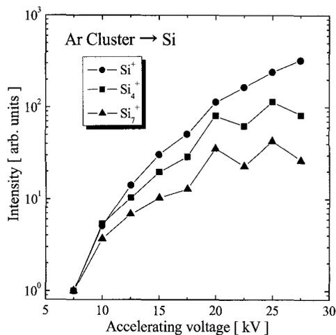
Fig. 3. Accelerating voltage dependence of relative secondary-ion yields per incident ion under Ar cluster ion bombardment.
