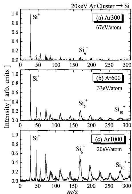
Fig. 4. Size dependence of secondary-ion spectra of Si obtained under the incidence of 20keV (a)  $\text{Ar}_{300}$ , (b)  $\text{Ar}_{600}$  and (c)  $\text{Ar}_{1000}$ .
