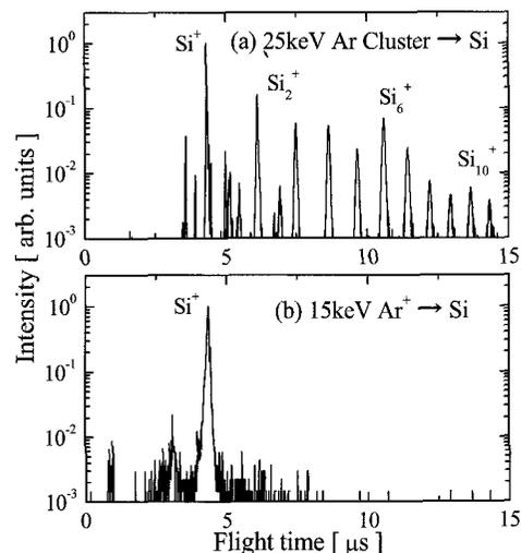
Fig. 2. Examples of TOF spectra of secondary ions for Si under (a) 25keV Ar cluster and (b) 15keV Ar monomer ion bombardment.
