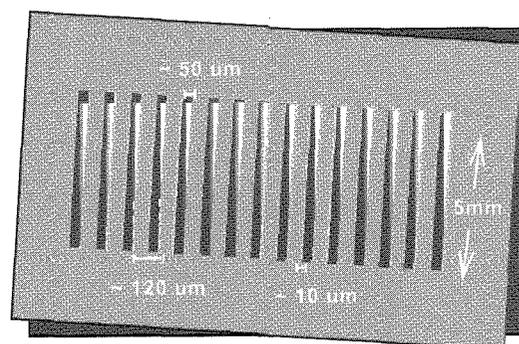
Fig.1. Schematic diagram of double mask to make an array of wedge-like apertures. The single mask has an array of rectangular apertures of 50  $\mu$ m width and 5 mm in length. As superimposing two masks at a little angle of 0.6 - 1 degree, wedge-like-aperture array is obtained. The minimum width is almost zero.
