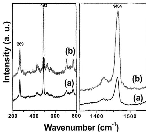
Fig.7, Raman spectra of (a) hexagonal  $C_{60}$  nanocrystals (b)  $C_{60}$  nanowhiskers
