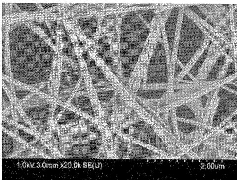
Fig.2, SEM image of platinum coated  $C_{60}$  nanowhiskers grown by the liquid-liquid interfacial precipitation method.
