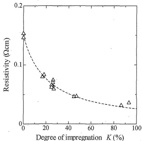
Fig. 6. Resistivity as a function of degree of impregnation.
