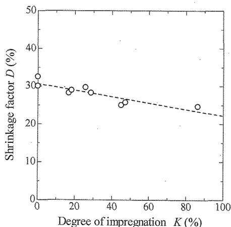
Fig. 3. Shrinkage factor as a function of degree of impregnation.
