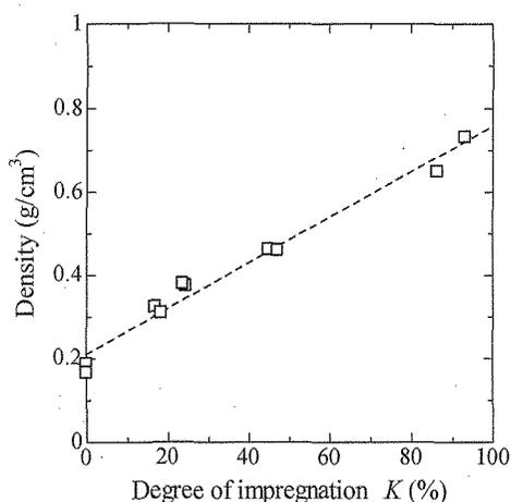
Fig. 7. Density as a function of degree of impregnation.
