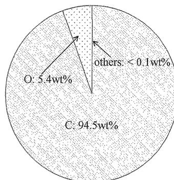
Fig. 4. Chemical compositions of woodceramics sheet (Degree of impregnation: 28.2 %).
