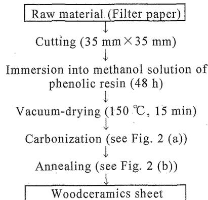
Fig. 1. Outline of manufacturing procedure for woodceramics sheet.
