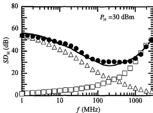
Fig. 6. The RF magnetic shielding degree  $SD_H$  for the first compound plate (solid circle), aggregated carbon plate (open squares), and ferrite plate (open triangles), as a function of frequency  $f$ , under a constant RF output power  $P_H$  of 30 dBm of the transmitting antenna. The solid line represents the sum of the values of  $SD_H$  for the aggregated carbon plate and the ferrite plate.
