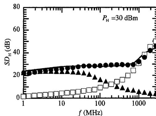
Fig. 7. Typical characteristics of RF magnetic shielding degree for the second compound plate (solid circles) constructed from aggregated carbon (open squares) and aggregated ferrite (solid triangles) plates, as functions of frequency  $f$ , under a constant RF output power  $P_H$  of 30 dBm of the transmitting antenna. The solid line represents the sum of the values of  $SD_H$  for the aggregated carbon and aggregated ferrite plates.
