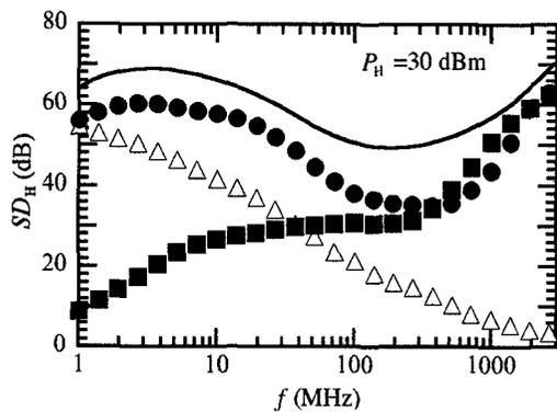
Fig. 5. The RF magnetic shielding degree  $SD_H$  of the superimposed plate (ferrite plate over the carbon plate, solid circles), the ferrite plate (open triangles) and the carbon plate (solid squares), as a function of frequency  $f$ , under a constant RF output power  $P_H$  of 30 dBm of the transmitting antenna. The solid line represents the sum of the values of  $SD_H$  for the individual carbon and ferrite plates.
