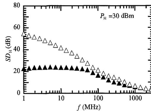
Fig. 4. Typical characteristics of the RF magnetic shielding degree  $SD_H$  as a function of frequency  $f$ , under a constant RF magnetic field power  $P_H$  of 30 dBm of the transmitting antenna. The open and solid triangles represent the results for the ferrite and aggregated ferrite plates, respectively.
