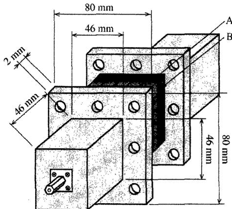
Fig. 2. Schematic diagram of the two metal cells used to measure the RF magnetic shielding effects. In this figure, A and B represent aggregated carbon and ferrite plates, respectively.
