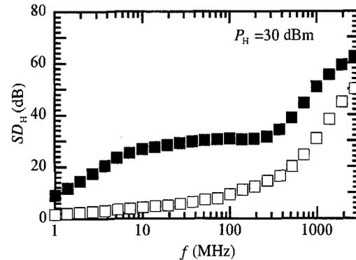
Fig. 3. The characteristics of  $SD_H$  for the carbon and aggregated carbon plates as a function of frequency  $f$ , under a constant RF output power  $P_H$  of 30 dBm of the transmitting antenna. The solid and open squares represent the results for the carbon and aggregated carbon plates, respectively.
