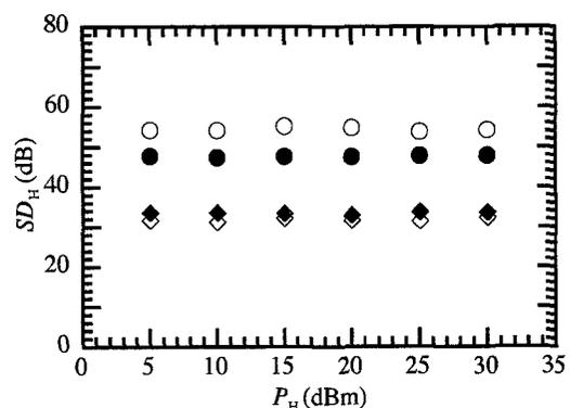
Fig. 8. Typical characteristics of  $SD_H$  for the first compound plate constructed from aggregated carbon and ferrite plates, as a function of RF output power  $P_H$  of the transmitting antenna. The open circles, solid circles, open diamonds, and solid diamonds represent the results for 1 MHz, 10 MHz, 100 MHz, and 1 GHz, respectively.
