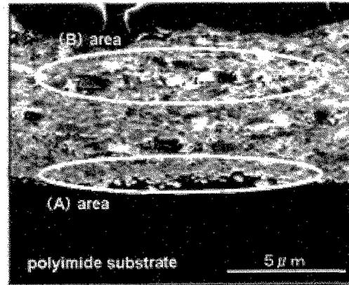
Fig. 7 The cross section image of Fe: Ferrite= 8:2 film
