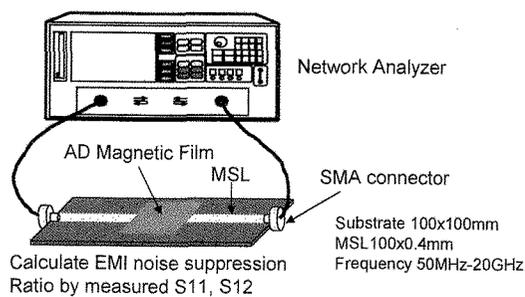
Fig. 2 An overview of experimental apparatus
