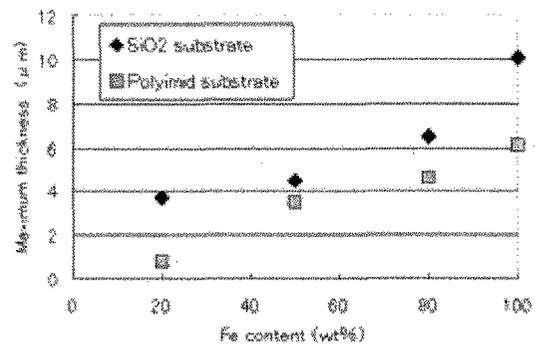
Fig. 3 The relationship between the maximum thickness of magnetic films and the amount of Fe
