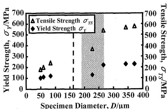
Fig.7 Relationship between specimen diameter and yield & tensile strengths. Dotted line indicates the position of average grain size of the sample. Cross-hatched pattern region indicates range of maximum grain size of the sample.
