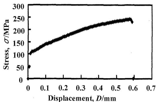
Fig.3 Stress-displacement curve obtained by tensile test of the micro-sized specimen with a diameter of 49  $\mu\text{m}$ .
