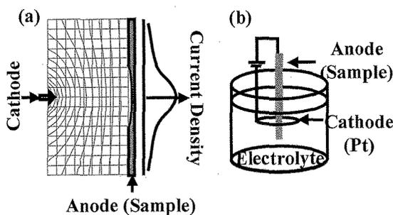
Fig.1 (a) Simulated electric potential distribution and (b) schematic illustration of the arrangements of electrodes in the electrolyte cell.
