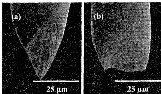
Fig.5 Scanning electron micrographs of fracture surface of the specimen with a diameter of 49  $\mu\text{m}$ . (a) Front view and (b) side view of the fracture surface.
