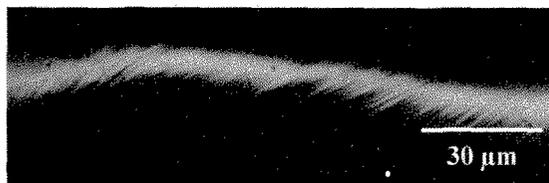
Fig.4 Laser micrograph of a deformed grain in single slips on the fracture specimen surface after tensile test.
