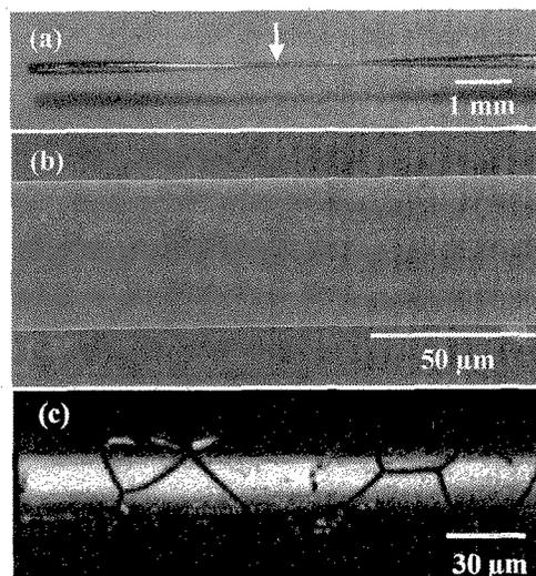
Fig.2 A micro-sized tensile specimen fabricated by electrolytic polishing. (a) Whole, (b) central point and (c) surface after 60 %  $\text{HNO}_3$  etching images of the specimen. A white arrow in Fig.2 (a) indicates the central position of ring-shaped cathode.
