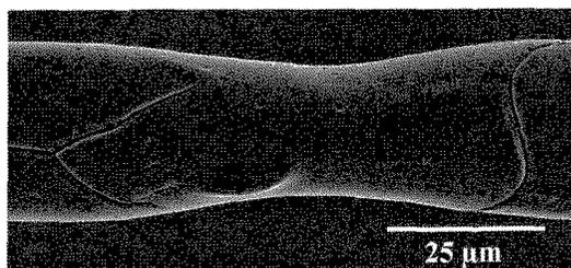
Fig.6 Scanning electron micrograph of necking deformation region away from fracture part after 60 %  $\text{HNO}_3$  etching.
