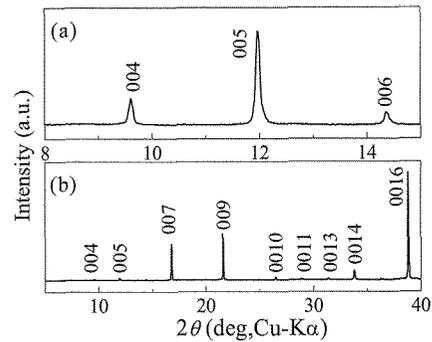
Fig.2. XRD patterns observed from the  $a$ - $b$  crystal surface of the BiT-PBTi crystals in the  $2\theta$  range of (a)  $8$ - $15^\circ$  and (b)  $5$ - $40^\circ$ .
