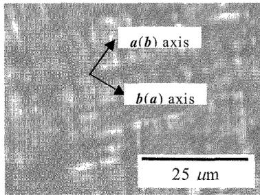
Fig. 1.  $90^\circ$  domain structure of BiT-PBTi in the  $a$ - $b$  plane.
