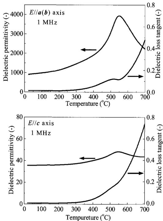
Fig.4. Temperature dependence of dielectric permittivity and loss tangent along the  $a(b)$  axis (a) and along the  $c$  axis (b) for the BiT-PBTi crystals.
