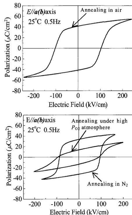
Fig.5 Polarization hysteresis loops of the BiT-PBTi crystals along  $a$  axis at 25°C.
