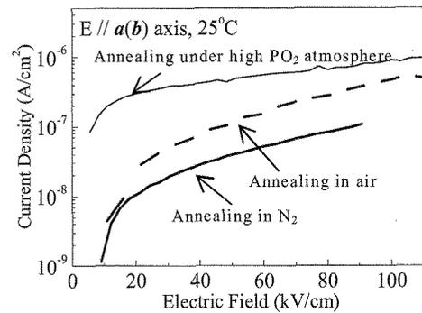
Fig.3. Leakage current properties of BiT-PBTi crystals along  $a$  axis at  $25^\circ\text{C}$ .
