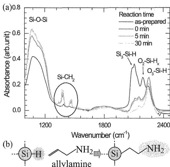
Fig.2. (a) Infrared absorption spectra of allylamine-treated PSi. The reaction time is shown in the figure. (b) Schematic illustration of surface modification by allylamine.
