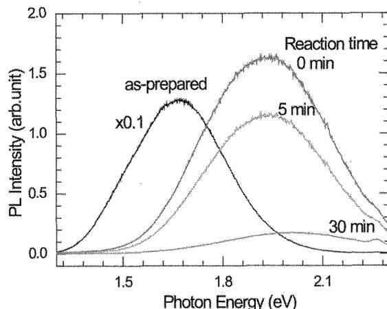
Fig.3 PL spectra of as-prepared PSi and allylamine-treated PSi with various reaction time in water.
