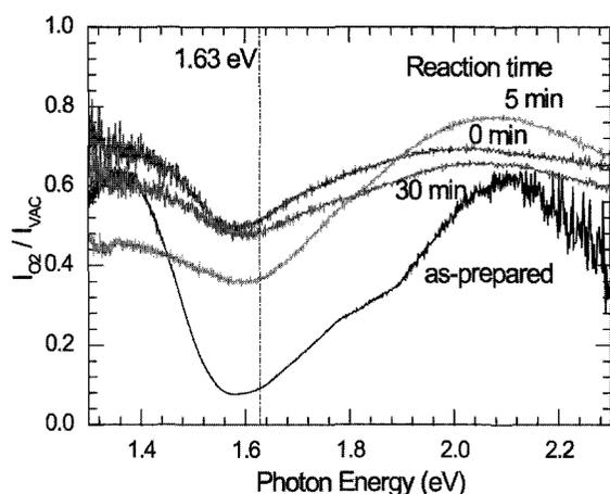
Fig.4. PL spectra taken in  $O_2$  atmosphere divided by that in vacuum ( $I_{oxygen}/I_{vac}$ ) at 150 K. The reaction time is shown in the figure.
