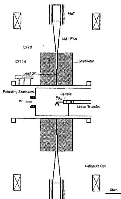
Fig. 2. Layout of the Ps-TOF spectrometer.
