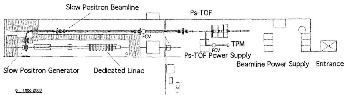
Fig. 1. The Slow Positron Facility. The facility consists of a dedicated 50 MeV linac, the Slow Positron Generator, the Slow Positron transport line and the Ps-TOF spectrometer.
