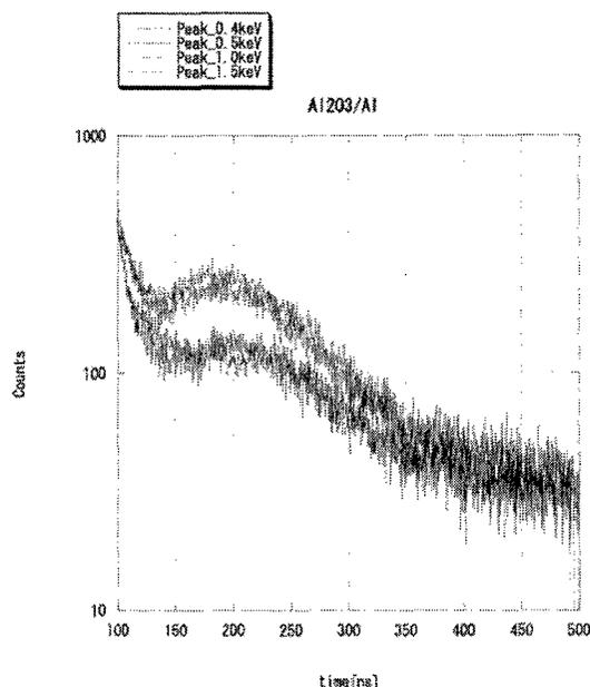
Fig. 3. Obtained Ps-TOF spector of  $Al_2O_3/Al$  with different implantation energy of positrons.
