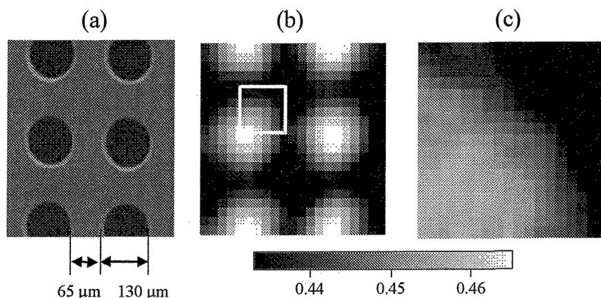
Fig. 4. (a) SEM image of the stainless mesh. (b) The spatial distribution of S parameter with the scan area of  $400 \times 400 \mu\text{m}$ . (c) The spatial distribution of S parameter with the scan area of  $80 \times 80 \mu\text{m}$  which corresponds to the square in (b).
