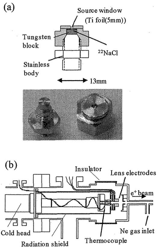
Fig. 2. Schematic drawings of (a) the positron source capsule and (b) the positron gun. The source is installed on the top of the cold head and cooled down to 4 K.
