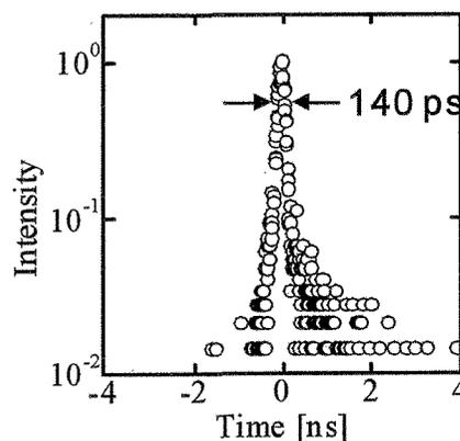
Fig. 5. The time structure of the bunched positron beam.
