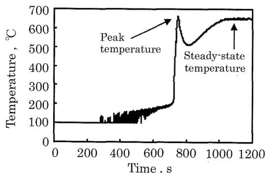
Fig. 3 Change in temperature of 10Cu powders (compacted mass: 0.8 g) during microwave irradiation.
