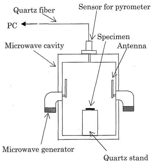
Fig. 1 Schematic diagram of the microwave irradiation test.
