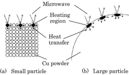
Fig. 9 Schematic illustration of microwave heating.
