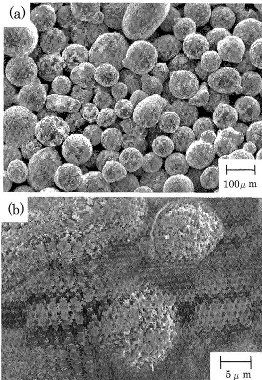
Fig. 5 SE images of 100Cu powder (compacted mass: 0.4 g) after microwave irradiation.
