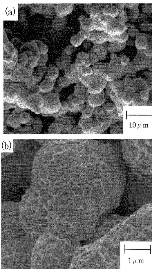
Fig. 4 SE images of 10Cu powder (compacted mass: 0.8 g) after microwave irradiation.
