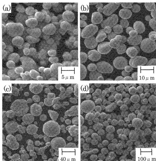
Fig. 2 SE images of the Cu powders used. (a) 5Cu, (b) 10Cu, (c) 45Cu and (d) 100Cu.
