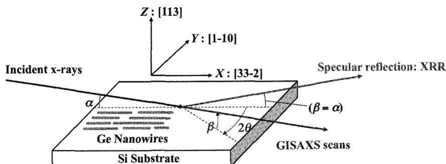
Fig. 1. The schematic of geometry of the measurements and orientation of Si substrate. The measurements were performed at the BL13XU beamline of the SPring-8 synchrotron facility.
