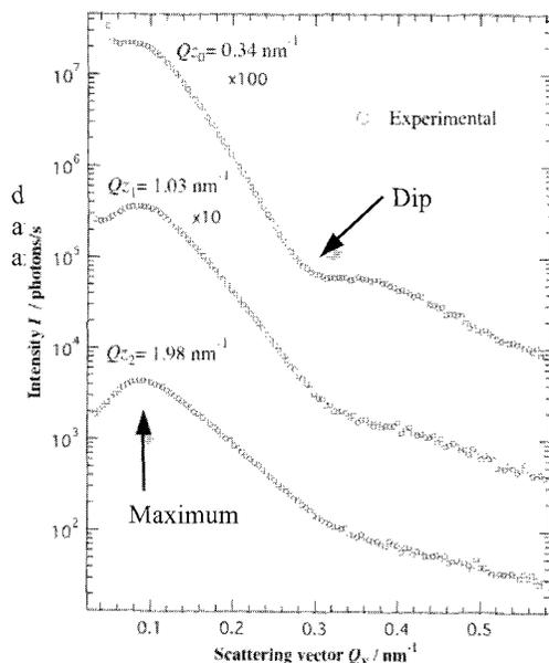
Fig. 3. Experimental GISAXS curves at the three  $Q_z$  positions. They have peaks at  $Q_y = 0.09\text{ nm}^{-1}$  and dips at  $Q_y = 0.30\text{ nm}^{-1}$ .
