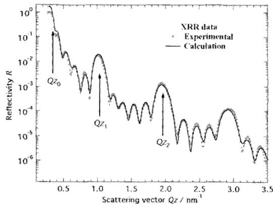
Fig. 2. Observed (circle) and calculated (solid line) XRR curves for analyzing the stacking structure. GISAXS measurements were performed at the three  $Q_z$  positions indicated by the arrows.
