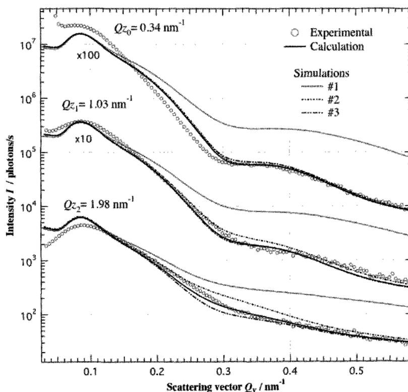
Fig. 4. Experimental (circle) and calculated (solid line) GISAXS curves at the three  $Q_Z$  positions. The additional three simulations (broken lines) are carried out for comparison. The meaning of each simulation is described in the text.
