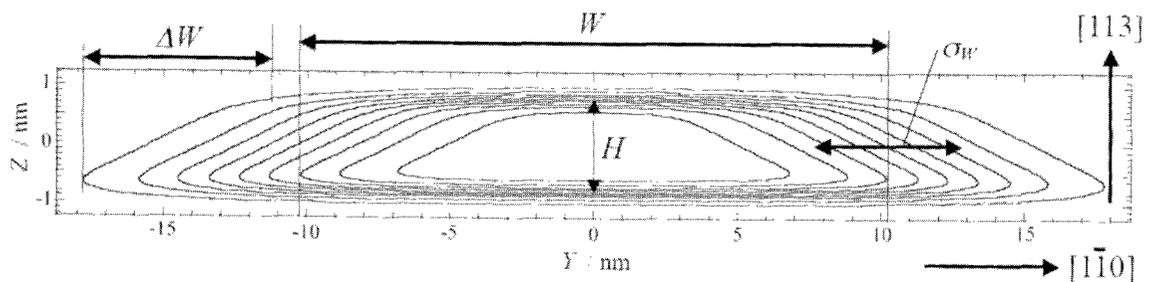
Fig. 5. Contour map of the Ge fraction of the nanowire in the  $(3\bar{3}2)$  plane. The  $Z$ -direction scale is elongated by two times as a matter of convenience. Interdiffusion is remarkable at the sides of the nanowires and facets are clearly seen.
