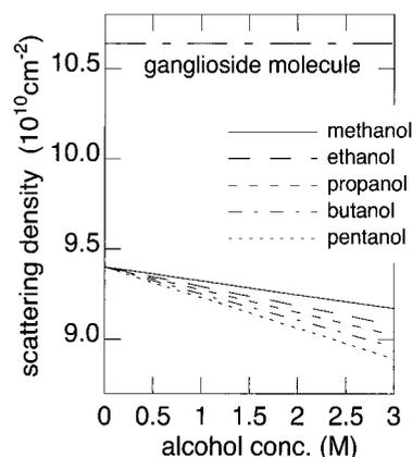
**Fig. 6.** Variation of the scattering density of alcohol-water binary solvent depending on alcohol concentration. The value of ganglioside molecule without hydration is also shown.
