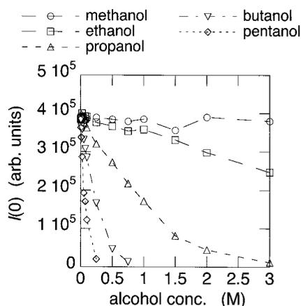
**Fig. 5.** Zero-angle scattering  $I(0)$  depending on alcohol concentration, which was obtained by the extrapolation of the Guinier equation.  $I(0)$  values are normalized by the expected changes of the contrasts depending on alcohol concentrations obtained from Fig. 6.
