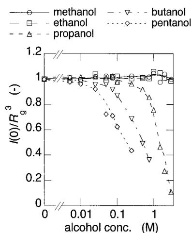
**Fig. 7.** Alcohol concentration dependence of zero-angle scattering  $I(0)$  normalized by  $R_g^3$ , which was obtained from depending on  $\lambda$ , which was obtained by Figs. 4 and 5.
