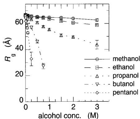
**Fig. 4.** Radius of gyration  $R_g$  depending on alcohol concentration. The lines show the least-square-fitted ones.
