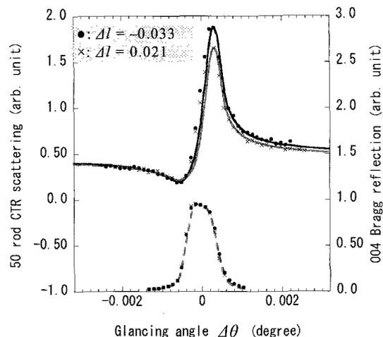
Fig. 3. An example of experimentally obtained modulation profiles. The abscissa is the deviation of the incidence angle from the center of the 004 Bragg reflection (denoted by  $\Delta\theta$ ). Filled circles and crosses correspond to experimentally obtained data, and solid and broken lines does to the calculated curves fitted to the experimental data.
