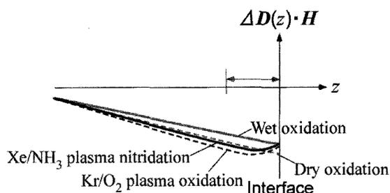
Fig. 4. Depth profiles of strain fields under the Si<sub>3</sub>N<sub>4</sub>/Si(001) interface (black solid line), where  $z$  represents the depth and  $\Delta D(z)$  is the sum of displacements defined in Fig. 2. For comparison some results of other oxidation processes are shown: gray solid and gray broken lines are the displacements induced by the wet and dry oxidations at 900 °C, and black broken line is that by the Kr/O<sub>2</sub> plasma oxidation at 400 °C.
