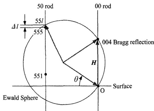
Fig. 1. Illustration of diffraction condition where intensity of CTR scattering is modulated by the excitation of the 004 Bragg reflection. The parameter  $l$  is the momentum transfer perpendicular to the surface, and  $\Delta l$  is the deviation of  $l$  from the 555 Bragg point.
