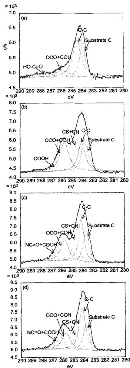
**Figure 2.** The XPS spectra of the substrates; (a) gold (b) SAM, (c) monomeric, and (d) dendritic. The changes by sugar-dendrimer immobilization was indicated by the allows, suggesting the density change of the sugar group.
