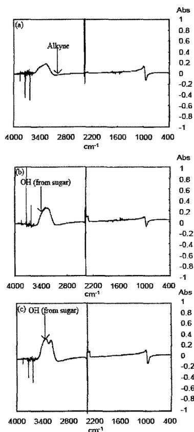
**Figure 1.** The FTIR-RAS spectra of the substrates; (a) SAM, (b) monomeric, and (c) dendritic. The changes by dendritic sugar immobilization was indicated by the allows, suggesting the density change of the sugar group.
