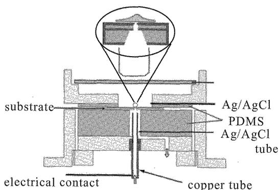
Fig.2 Schematic view of planar ion channel biosensor device with SOI substrate.
