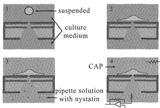
Fig. 4 Steps in planar ion channel current recording
