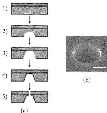
Fig. 1 (a) Schematic of sensor chip fabrication; (b) SEM image of micropore fabricated by FIB milling (scale bar 0.5  $\mu\text{m}$ ).
