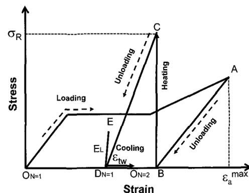
Fig.1 A schematic drawing of thermomechanical cyclic test.
