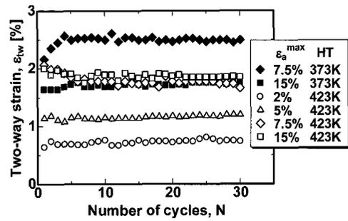
Fig.4 Variation of two-way strain with number of cycles.
