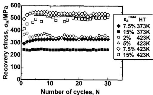
Fig.7 Variation of recovery stress with number of cycles.
