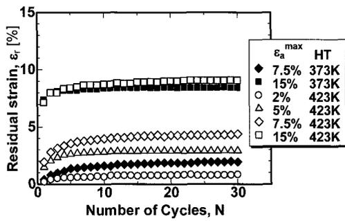
Fig.2 Variation of residual strain with number of cycles.
