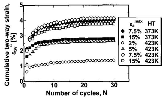
Fig.5 Variation of two-way strain with number of cycles.
