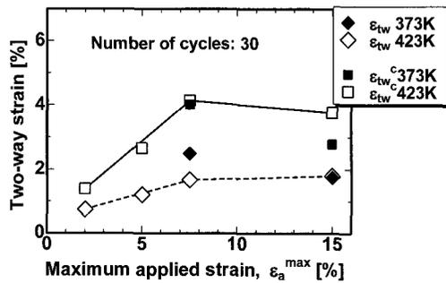
Fig.6 Relationship between two-way strain and maximum applied strain.
