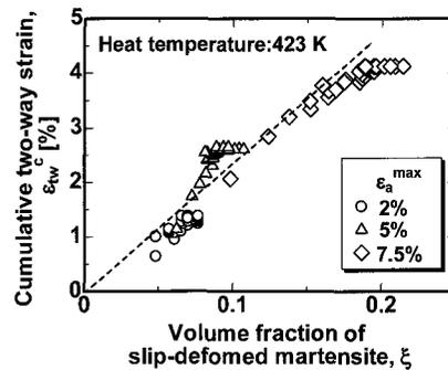
Fig.9 Relationship between cumulative two-way strain and volume fraction of slip-deformed martensite.
