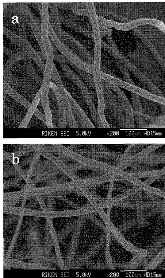
Fig.2 SEM photographs of non-implanted PTFE fiber (a) and Ar<sup>+</sup> ion implanted PTFE fiber (b).
